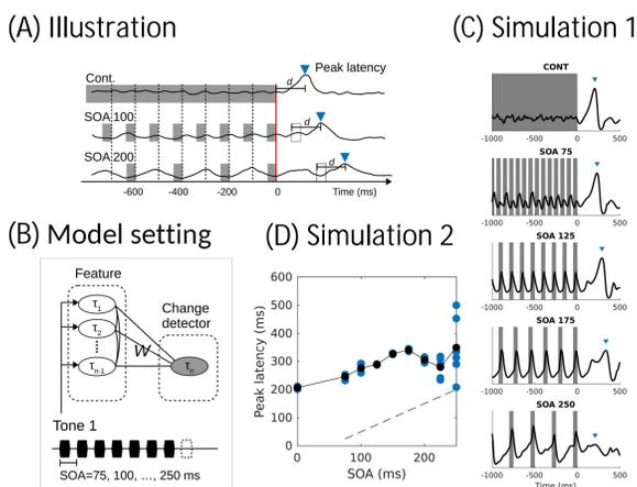
Fig. 4. (A) The OSR peak latency is a constant delay plus the SOA. (B) The feature columns have different time constants  $\tau_i$  so that the periodicity (i.e. SOA of stimuli) is kept in sustained resonance. The change detector responds to a sudden change in periodicity. (C) Simulated temporal responses. (D) Simulated OSR latencies show temporal expectancy.
