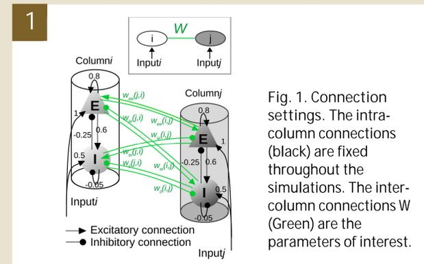
Fig. 1. Connection settings. The intra-column connections (black) are fixed throughout the simulations. The inter-column connections  $W$  (Green) are the parameters of interest.
