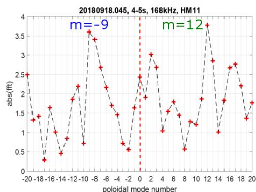
Fig. 3: Experimentally observed poloidal mode numbers for PID 20180918.045 during the time period of 4-5s. The mode number analysis was done using the SSI-method on the measured data of the poloidally arranged Mirnov coils in HM11.
