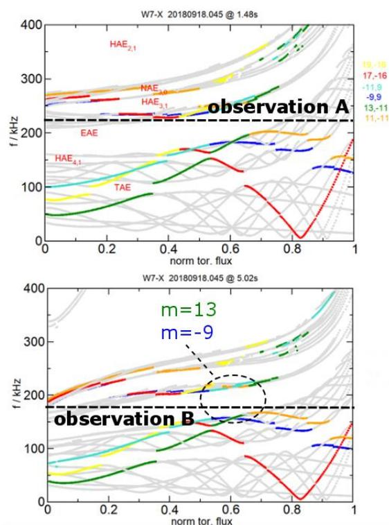
Fig. 2: Alfvén continua calculated using CONTI for PID 20180918.045 at two time points 1.48s (top) and 5.02s (bottom). Expected poloidal mode numbers are indicated for a direct comparison with experimental results ( $n = 1$  mode family).
