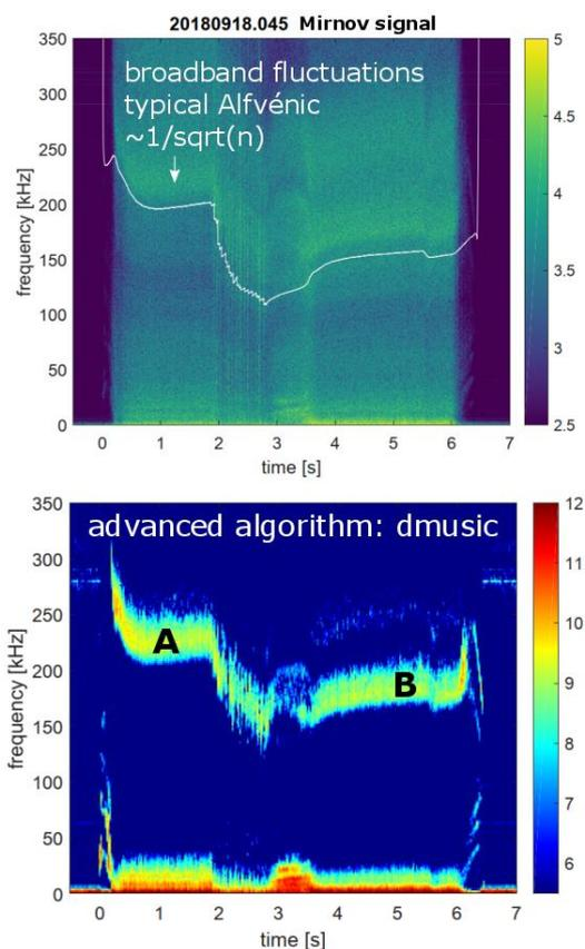
Fig. 1: *top*: typical frequency spectrum measured by a selected Mirnov coil; *bottom*: same data as above, but calculated using the advanced spectral analysis tool DMUSIC.
