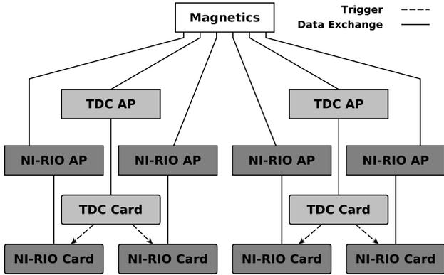
Figure 2: Illustration of the internal AP structure of the DCS satellite for the new magnetics on ASDEX Upgrade. The APs are indicated by the grey rectangles, the hardware is indicated by the grey boxes with rounded corners.
