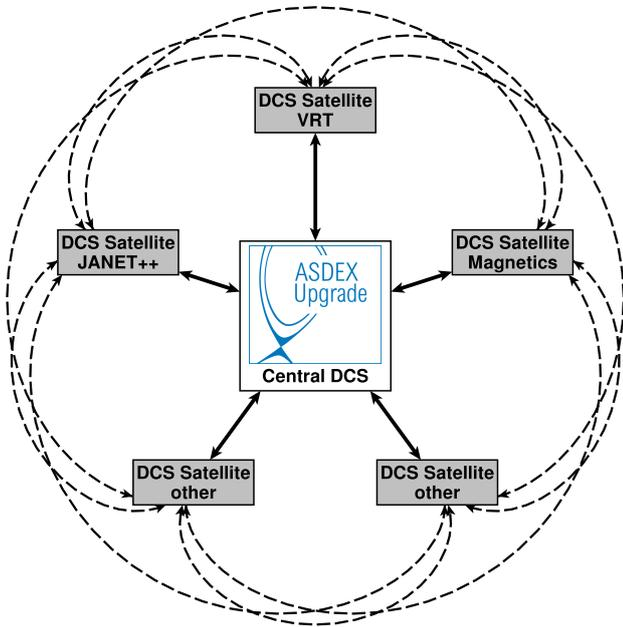
Figure 1: Illustration of DCS satellites communication with central DCS. The real time data and configuration communication is shown as bold arrows, the real time data only communication is shown as dashed arrow. Offline data storage is handled by the data management system at ASDEX Upgrade [17] and is not illustrated in this figure.
