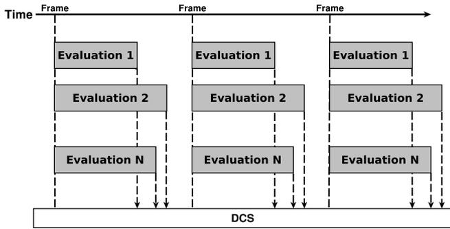
Figure 5: Illustration of the VRT evaluation timing. All evaluations for a camera are executed when a new frame has been acquired. The result for each evaluation is send to DCS as soon as it becomes available.
