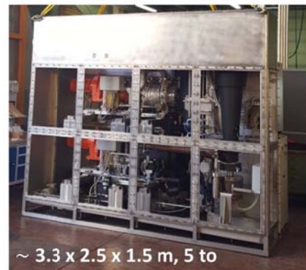
Fig. 10. Mercury based vacuum pump train for JET (during transportation to the commissioning facility).
