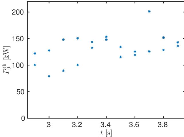
**Figure 10.** Gyrotron power threshold,  $P_0^{\text{th}}$ , versus  $t$  in ASDEX Upgrade discharge 28286.  $P_0^{\text{th}} \sim 100$  kW in the shown part of the discharge and generally below the nominal gyrotron power,  $P_0 = 200$  kW.
