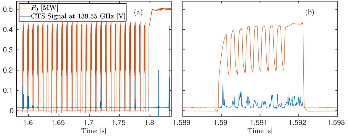
**Figure 5.4** –  $P_0$  pulses with analog modulations and CTS signal in ASDEX Upgrade #36583. Pane (a) shows an overview of the pulses and the beginning of the continuous wave phase after the pulses; pane (b) shows the signals during pulse #1.
