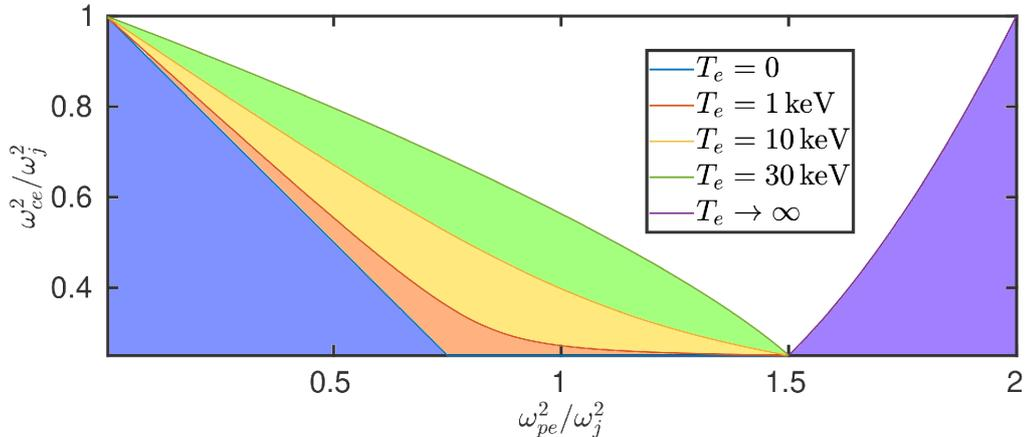
**Figure 2.2** – Electron Bernstein wave CMA-like diagram where  $\ell_{Te,j}^2 > 0$ . No propagating EBWs exist in the blue or purple shaded regions at any  $T_e$ . For  $T_e = 1$  keV, no propagating EBWs additionally exist in the orange shaded region, for  $T_e = 10$  keV the yellow shaded region is added to the region with no propagation EBWs, and for  $T_e = 30$  keV the green shaded region is finally added.
