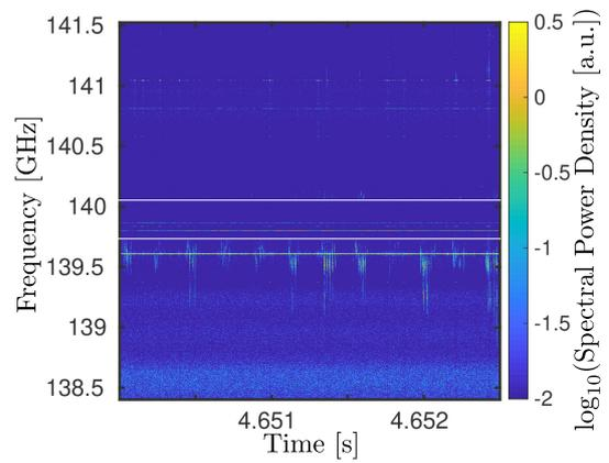
**Figure 5.15** – Fast CTS signal near 140 GHz during a rotating magnetic island in ASDEX Upgrade #35527. The white lines mark the edges of the notch filter around the gyrotron lines. Spikes occur with a repetition rate determined by the mode frequency.
