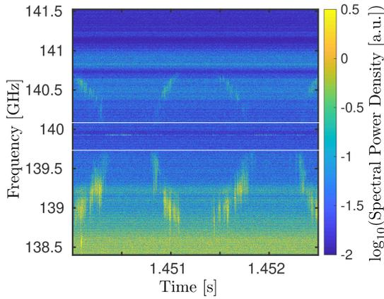
**Figure 5.14** – Fast CTS signal near 140 GHz during a rotating magnetic island in ASDEX Upgrade #35186. The white lines mark the edges of the notch filter around the gyrotron line. Spikes occur with a repetition rate determined by the mode frequency.
