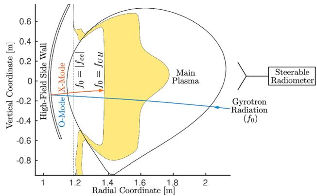
**FIG. 1.** Schematic of the experimental setup in AUG discharge 34575. No propagating X-mode exists in the shaded region.
