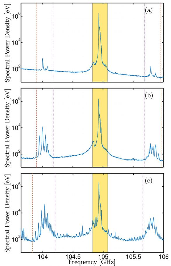
**FIG. 4.** Mean spectra recorded by the steerable radiometer in AUG discharge 34575 at  $B_t = -2.53$  T (a),  $B_t = -2.48$  T (b), and  $B_t = -2.44$  T (c). The shaded areas indicate the stopband of the notch filter near  $f_0$ , where the calibration is uncertain. The dashed lines indicate the most unstable modes according to Ref. 26; the dotted lines indicate  $f_0 \pm f_{LH}$ .
