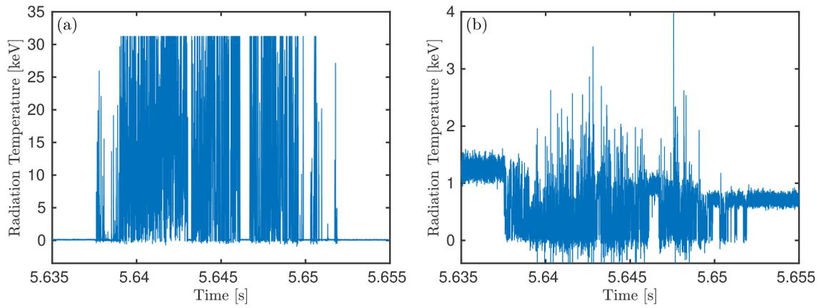
**Figure 5.25** – Degradation of ECE mixer during central PDI in ASDEX Upgrade #36149. Pane (a) shows the signal from a channel around 75.5 GHz; pane (b) shows the signal from a channel around 87.9 GHz.
