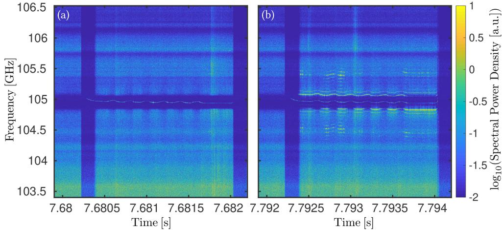
**Figure 1.2** – Mixing of ECRH and ICRH waves in ASDEX Upgrade #34195. In pane (a), no ICRH power is injected, leading to a single line from the CTS gyrotron around 105 GHz. In pane (b), ICRH power with a frequency of 55.1 MHz is injected, leading to side bands separated by the ICRH frequency around the CTS gyrotron line. The low spectral power density around 105 GHz is due to the CTS notch filter; the overall low spectral power during switch on/off of the gyrotron is due to the CTS pin-switch.
