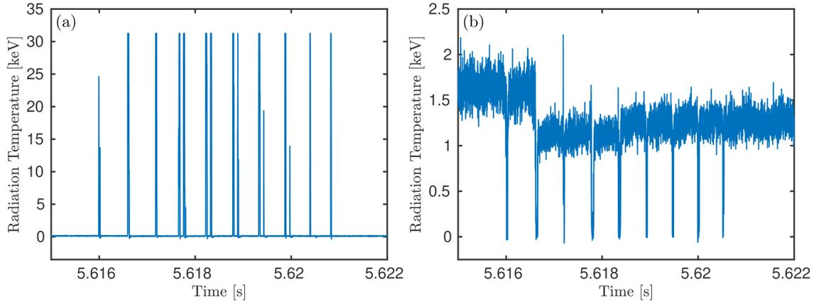
**Figure 5.13** – Degradation of ECE mixer during a rotating magnetic island in ASDEX Upgrade #35939. Pane (a) shows the signal from a channel around 75.5 GHz; pane (b) shows the signal from a channel around 87.9 GHz.
