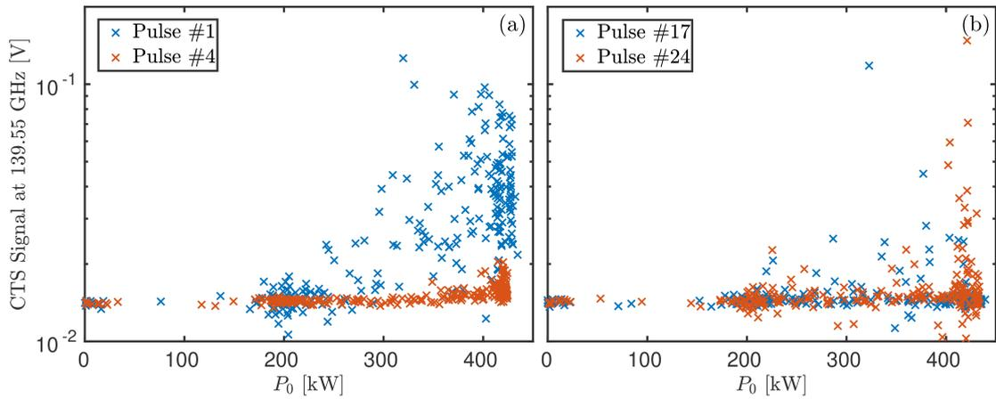
**Figure 5.5** – Plot of  $P_0$  versus the CTS signal at 139.55 GHz to determine  $P_0^{\text{th}}$  in ASDEX Upgrade #36583. Pane (a) shows pulses before the start of the ELM phase, while pane (b) shows pulses in which ELM crashes occur.
