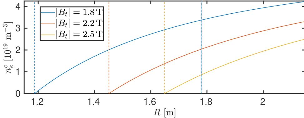
**Figure 5.1** –  $n_e^c$  at different  $B_t$  for a 140 GHz pump wave in ASDEX Upgrade ( $R_0 = 1.65$  m and  $a = 0.5$  m). The solid lines mark  $n_e^c$ , the dashed vertical lines mark the second-harmonic ECR, and the dotted vertical line marks the third-harmonic ECR for  $|B_t| = 1.8$  T.
