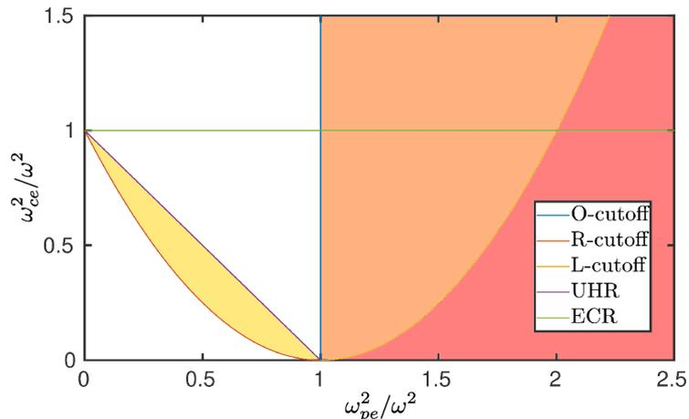
**Figure 2.1** – CMA diagram. No propagating X-mode exists in the yellow shaded region, no propagating O-mode exists in the orange shaded region, and neither the O-mode nor the X-mode is propagating in the red shaded region.
