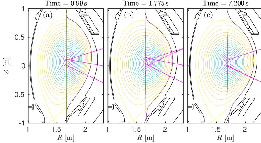
**Figure 5.2** – Plasma scenarios with spikes during ELMs in ASDEX Upgrade: #35676 (a), #36583 (b), and #33616 (c). Green lines are the 140 GHz second-harmonic ECR, magenta lines are gyrotron beams, and purple lines are the 70 GHz warm UHR. Pane (a) and (c) appeared in [20].
