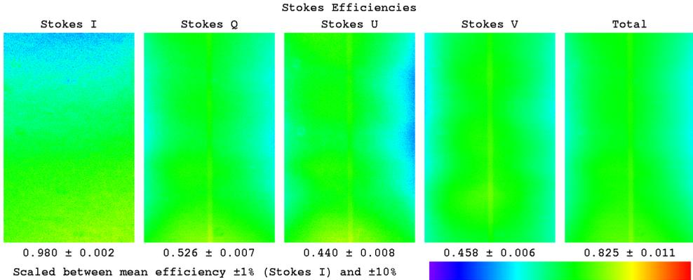
**Figure 3.** Field dependency of measured polarimetric efficiencies for 630 nm (single measurement).
