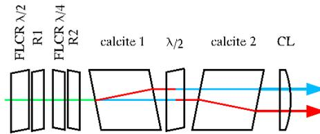
**Figure 1.** Scheme of the polarimeter. The additional retarders are marked by R1 and R2. The cylindrical lens is marked by CL.
