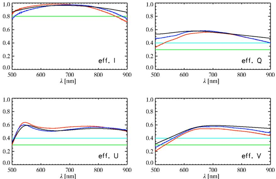
**Figure 2.** Expected (*black*) and measured polarimetric efficiencies for the GFPI-polarimeter (*red and blue*). The horizontal lines indicate the thresholds of 0.3 and 0.4
