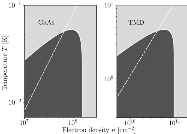
FIG. 7. Melting curves of (left) GaAs and (right) monolayer TMD systems according to the Lindemann criterion. The dark areas indicate the onset of WC electron lattices, obtained for  $N = 20$  electrons. The dashed line indicates  $k_B T = \epsilon_F$ .
