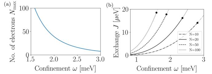
FIG. 2. Spin coupling and system size. (a) Maximum number of electrons as a function of  $\omega$  such that  $n < n_{\text{cr}}$ . (b) Coupling constant  $J$  as a function of the confinement  $\omega$  for different particle numbers  $N = 10$  (dash dotted),  $N = 20$  (solid),  $N = 50$  (dashed),  $N = 100$  (dotted). Black dots: Maximum frequency  $\omega$  for given  $N$  such that  $n < n_{\text{cr}}$ .
