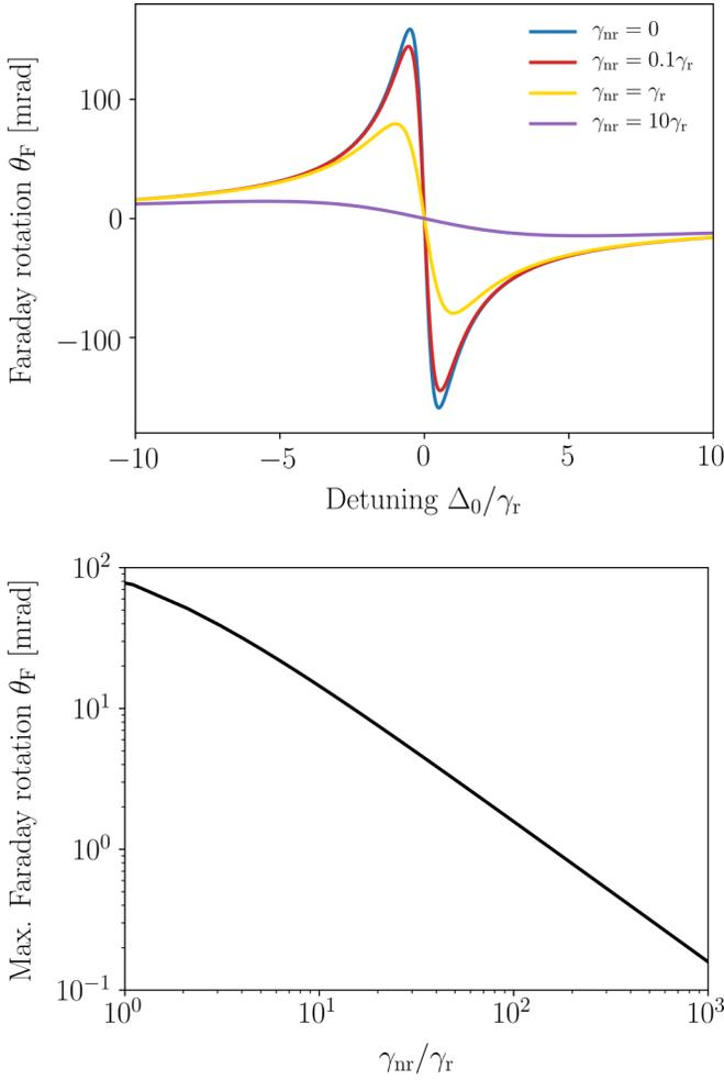
FIG. 10. Faraday rotation for different  $\gamma_{nr}$  and the same numerical parameters as in Fig. 3 at  $N_{\uparrow} = 15$ ,  $N_{\downarrow} = 5$ . Also shown is the maximum Faraday signal as a function of  $\gamma_{nr}/\gamma_r$ .
