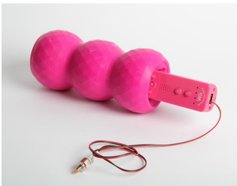
Figure 6. The wireless prototype. The cable, connecting our external custom synchronization button to the Wii Remote, can be hidden inside the Kong toy once the synchronization is accomplished.
