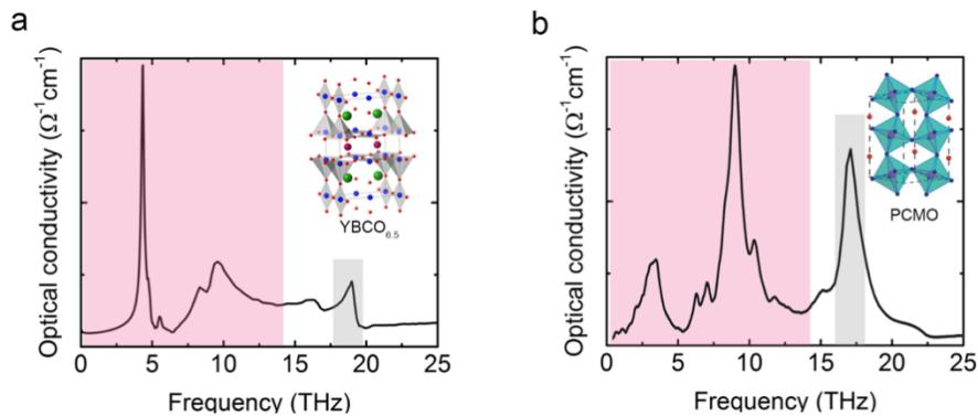
**Figure 1.12.** Optical conductivity along  $c$  direction in (a)  $\text{YBa}_2\text{Cu}_3\text{O}_{6.5}$  and (b)  $\text{Pr}_{0.7}\text{Ca}_{0.3}\text{MnO}_3$ . The phonons investigated previously are highlighted in grey. Low energy phonons in the THz-gap range are highlighted in red. Insets, crystal structures for  $\text{YBa}_2\text{Cu}_3\text{O}_{6.5}$  and  $\text{Pr}_{0.7}\text{Ca}_{0.3}\text{MnO}_3$  [1].
