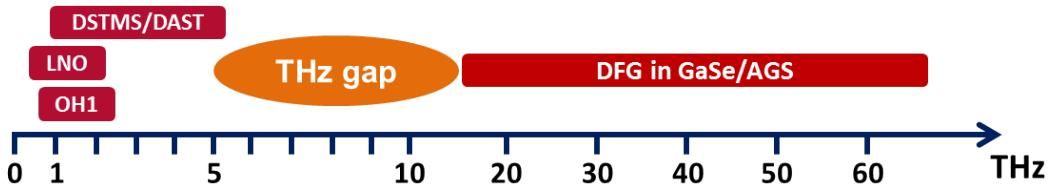
**Figure 2.7. General table-top techniques of intense THz pulses generation.** Below 5 THz, Optical rectification are widely used in ferroelectric material (e.g. LiNbO<sub>3</sub>) and large piece of organic crystals (OH1, DSTMS, DAST). Above 15 THz, frequency mixing using near-infrared pulses can be exploited in semiconductor emitters like GaSe, AgGaS<sub>2</sub>. Efficient light source in the “THz gap” is still on demand.
