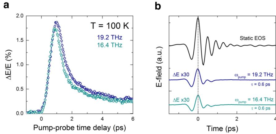
**Figure 4.12.** (a) Pump-induced changes at the peak of the THz probe electric field as a function of pump-probe time delay, measured in YBCO<sub>6.5</sub> at  $T = 100 \text{ K}$  (below  $T_c$ ) for narrowband excitation at 16.4 THz and 19.2 THz excitations. (b) The static reflected probe electric field and corresponding pump-induced electric field changes for 19.2 THz and 16.4 THz at pump-probe delay  $\tau = 0.6 \text{ ps}$ .
