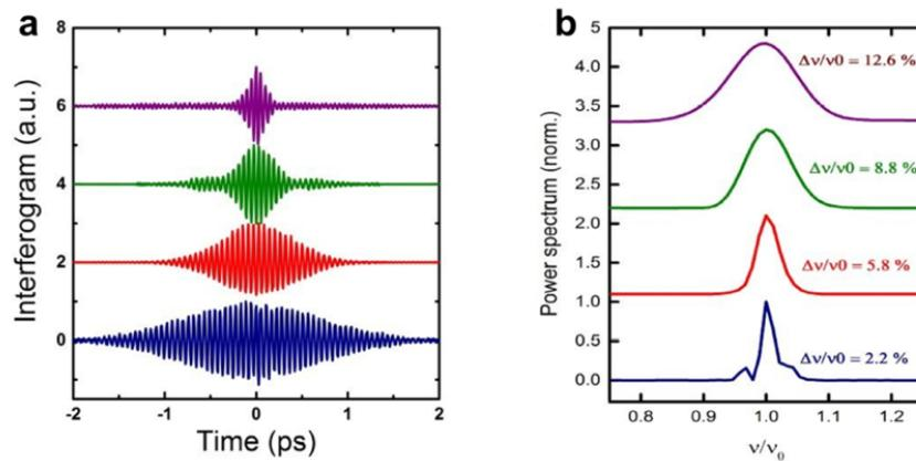
**Figure 2.18.** (a) Interferograms for the THz fields generated by using near-IR pulses with different duration. (b) The corresponding relative bandwidth  $\Delta v/v_0$  (FWHM) of the THz fields shown in (a).
