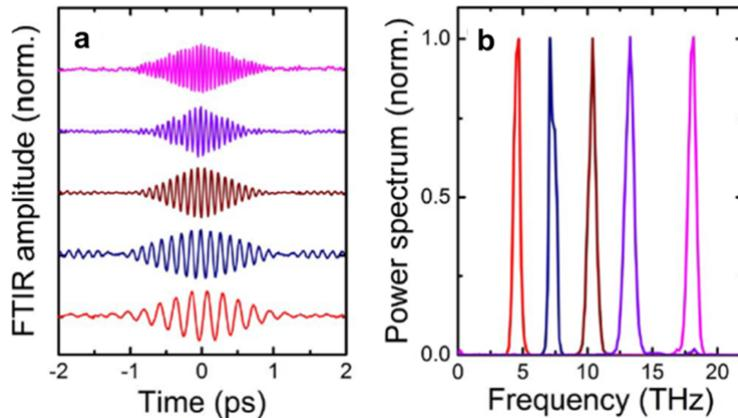
**Figure 2.17.** (a) Normalized FTIR interferograms and (b) the corresponding Fourier spectrum of the THz fields, tuned by changing the difference frequency between the two linearly-chirped near-IR pulses.
