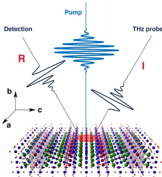
**Figure 4.5.** THz pump - THz probe geometry in the  $\text{YBCO}_{6.5}$  experiment. The THz pump pulses, polarized along the  $c$ -axis, were shone onto the  $ac$ -plane surface of the  $\text{YBCO}_{6.5}$  sample. Broadband THz pulses with incident angle at 30 degrees, also polarized along the  $c$ -axis, were used to probe the pump-induced changes in the  $\text{YBCO}_{6.5}$  optical response functions. “I” and “R” stand for “incident” and “reflected” pulse, respectively.
