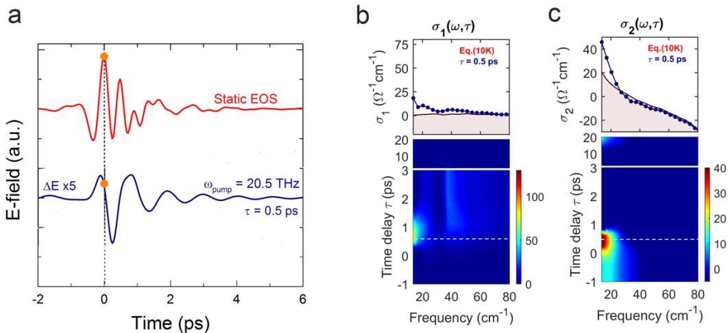
**Figure 4.19.** (a) Stationary reflected probe electric field and corresponding pump-induced electric field changes for 20.5 THz narrowband excitations at a pump-probe delay  $\tau = 0.5 \text{ ps}$ . (b-c) Frequency- and time-delay-dependent pump-induced optical conductivity measured after narrowband excitation at 20.5 THz ( $T = 10 \text{ K}$ , below  $T_c$ ). The white dashed lines indicate the pump-probe time delay  $\tau = 0.5 \text{ ps}$ .
