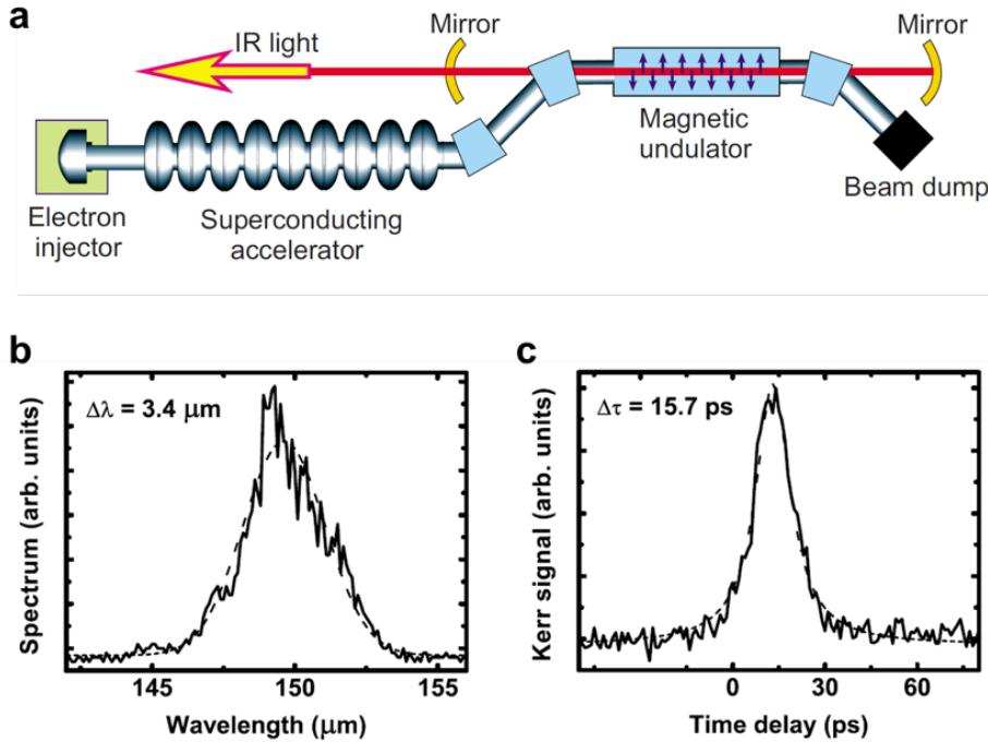
**Figure 2.1.** (a) Schematic view of the free-electron laser in the FZD. (b) Measured spectrum of the FEL at 150- $\mu\text{m}$  wavelength. (c) The Electro-optic sampling of the free electron laser pulses in a ZnTe crystal. The FWHM of the Kerr signal reveals a pulse duration of  $\sim 16 \text{ ps}$ . Taken from Ref. [40].
