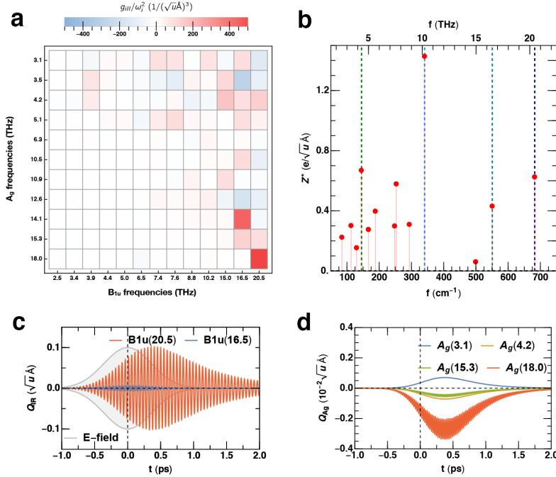
**Figure C.1.** (a) Third-order anharmonic coupling coefficients of the type  $Q_{Ag} Q_{IR}^2$  for all  $B_{1u}$  and  $A_g$  modes. (b) Mode effective charges for the polar  $B_{1u}$  modes of the  $\text{YBa}_2\text{Cu}_3\text{O}_{6.5}$  ortho-II structure. (c) Oscillations of two  $B_{1u}$  modes at 16.5 and 20.5 THz driven by a narrowband THz pulse at 20.5 THz (grey area). (d) Dynamics of the four  $A_g$  modes exhibiting stronger coupling to the 20.5-THz  $B_{1u}$  mode driven in (c).
