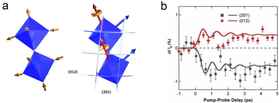
**Figure 1.4.** (a) Left: atomic motions of the  $E_u$  symmetry Mn-O stretching mode in  $\text{La}_{0.7}\text{Sr}_{0.3}\text{MnO}_3$ . Right: sketch of the nonlinearly driven Raman-active mode, the rotation of the O-octahedra is around an axis (red) perpendicular the [111] crystal axis. (b) Relative X-ray intensity changes of the (201) and (012) Bragg peaks induced by MIR excitation. Figures are taken from [25].
