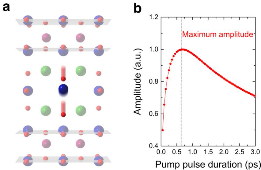
**Figure C.3.** (a) Atomic motion of the apical-oxygen mode in the O-deficient chain at 19.2 THz of YBCO<sub>6.5</sub> projected in *ac*-plane with CuO<sub>2</sub> layers highlighted in grey. (b) The simulated maximum amplitude of 19.2-THz mode by transform-limited MIR pulses with different pulse durations. The damping coefficient is extracted from the linewidth of the phonon. The dashed line indicates the best pulse duration of around 600 fs.
