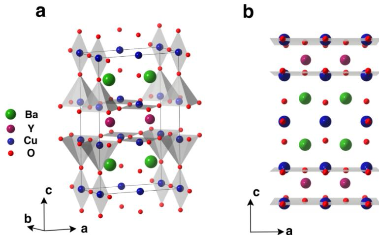
**Figure 4.1.** (a) Crystallographic unit cell of orthorhombic  $\text{YBa}_2\text{Cu}_3\text{O}_{6.5}$  (ortho-II). Bilayers of conducting  $\text{CuO}_2$  planes, stacked along the *c*-axis, forming the Josephson junctions. (b) Crystal structure projected in the *ac*-plane. The  $\text{CuO}_2$  layers highlighted in grey.
