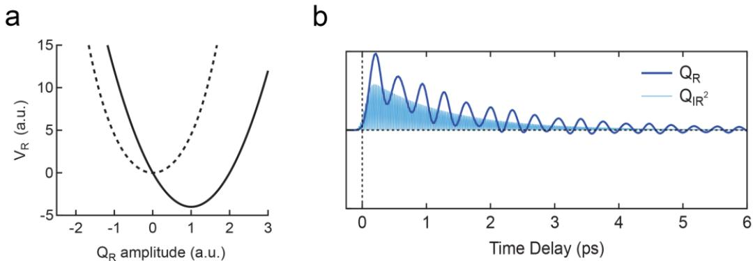
**Figure 1.1.** (a) Equilibrium energy potential (dashed curve) and the shifted potential through the cubic nonlinear coupling (solid curve) for the Raman mode. (b) Dynamics of the driving force (light blue) and the normal coordinate (dark blue) for the anharmonically coupled Raman mode [17].
