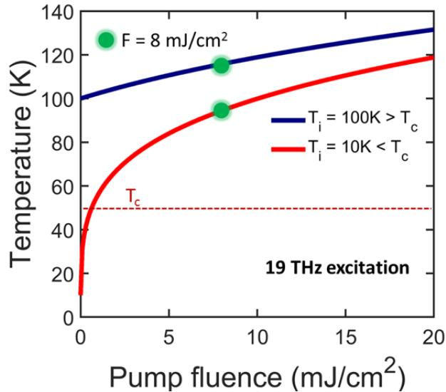
**Figure C.5.** Calculated final lattice temperature after electron-phonon thermalization as a function of pump fluence after 19 THz excitation in YBCO<sub>6.5</sub>. The red curve and blue curve are corresponding to different initial temperature at 10 K (superconducting) and 100 K (insulating), respectively. The red dashed line is superconducting transition temperature  $T_c$  at 52 K.
