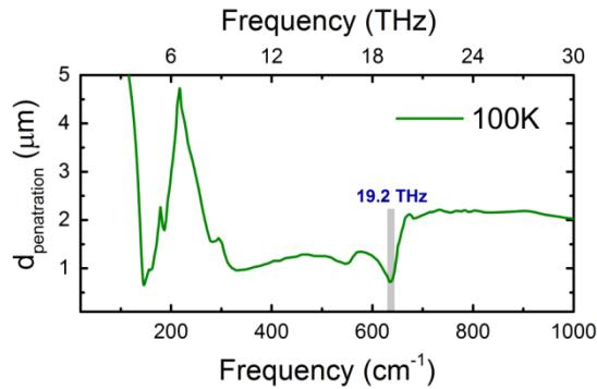
**Figure D.2.** Frequency-dependent penetration depth for the pump light wave along the  $c$ -axis in YBCO<sub>6.5</sub> at 100 K. The value for 19.2 THz is  $0.7 \mu\text{m}$ , which is highlighted in grey.
