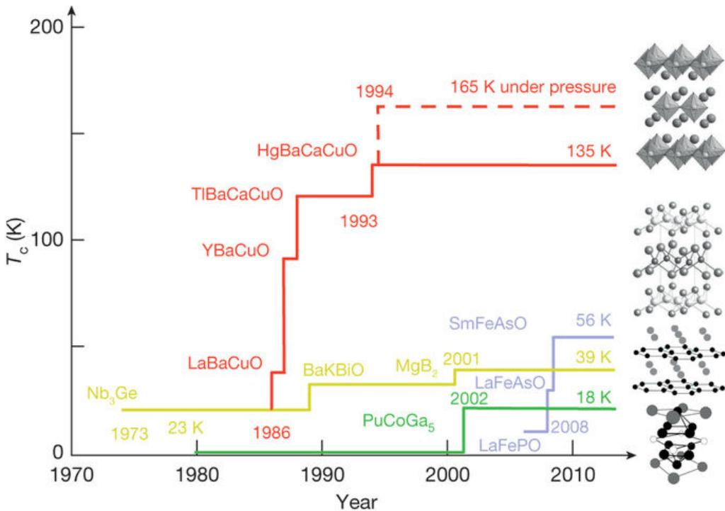
**Figure 3.4.** Superconducting transition temperatures versus year of discovery for various classes of superconductors. The images on the right are the crystal structures of representative materials. The timelines for conventional superconductors, heavy-fermions, cuprates, and iron-based pnictides are plotted in gold, green, red and light grey, respectively. Adapted from Ref. [117].
