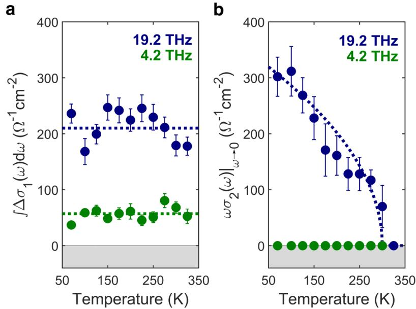
**Figure 4.16.** Temperature-dependent (a) dissipative response,  $\int \Delta\sigma_1(\omega)d\omega$ , and (b) superconducting-like response,  $\omega\sigma_2(\omega)|_{\omega\rightarrow 0}$ , measured for resonant narrowband excitation of the lowest-frequency (4.2 THz) and highest-frequency (19.2 THz) phonon modes. The dashed lines are guides to the eye [35].
