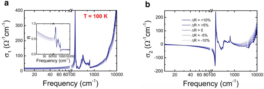
**Figure D.1.** (a) The real part of optical conductivity obtained from Kramer-Krönig transformation with  $\pm 5\%$  and  $\pm 10\%$  statistic error in the measured Reflectivity. Inset: Reflectivity with  $\pm 5\%$  and  $\pm 10\%$  statistic error in the measurement. (b) The imaginary part of optical conductivity.
