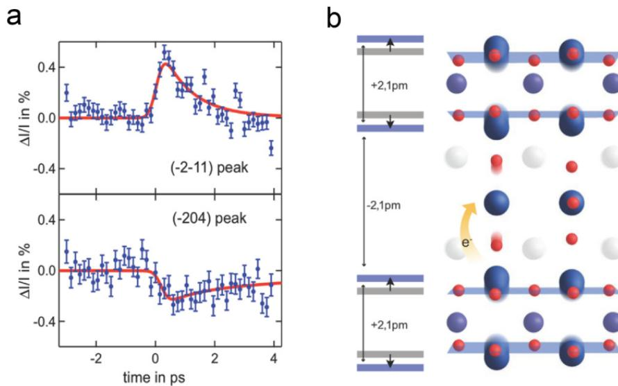
**Figure 1.11.** (a) Relative changes in the diffracted intensity of (-2-11) and (-204) Bragg peaks in  $\text{YBCO}_{6.5}$  following the MIR resonant excitation. (b) Sketch of the reconstructed transient crystal structure at the peak signal. The redistributed layer distance of the Josephson layers is evidenced. Adapted from [13].
