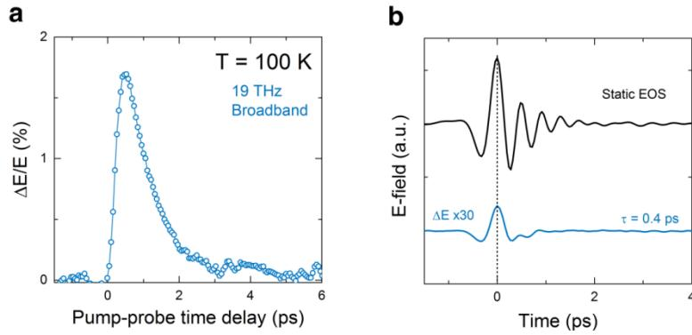
**Figure 4.10.** (a) Pump-induced changes at the peak of the THz probe electric field as a function of pump-probe time delay, measured in YBCO<sub>6.5</sub> at T = 100 K (> T<sub>C</sub>) for broadband 19 THz excitation. (b) Stationary reflected probe electric field and corresponding pump-induced electric field changes at  $\tau = 0.4$  ps time delay.
