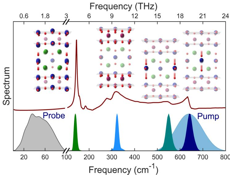
**Figure 0.3.** Top: Various optical vibration modes along the *c*-axis of YBa<sub>2</sub>Cu<sub>3</sub>O<sub>6.5</sub>. Middle: optical conductivity in the same direction. Bottom: Fourier spectrum of different generated THz pulses together with the broadband THz probe.
