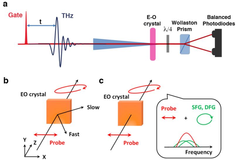
**Figure A.1.** (a) Schematic illustration of Electro-optic sampling. (b-c) Two different description of the birefringence in the Electro-optic sampling: (b) Pockels effect description and (c) frequency-mixing description. EO: electro-optic, SFG: sum frequency generation, DFG: difference frequency generation. (b-c) are adapted from Ref. [183]
