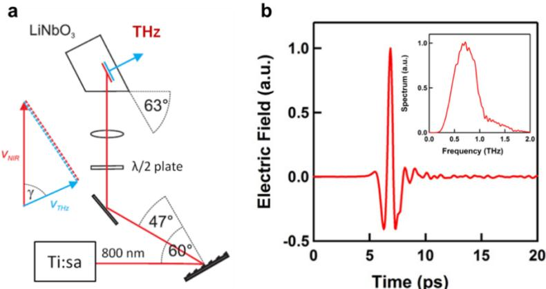
**Figure 2.4.** (a) The pulse front of near-infrared pulses at 800 nm generated from a Ti:sapphire laser amplifier is tilted by an angle of  $\gamma$  to fulfill the phase matching condition. The pulse front tilting is achieved by diffracting the beam off a grating at an incident angle of 60 degrees. (b) Characterization of the generated THz pulse via electro-optical sampling. Inset, the corresponding Fourier transform of the measured electric field.
