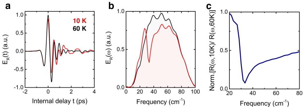
**Figure 4.17.** (a) Stationary electric field profile measured after reflection from  $\text{YBa}_2\text{Cu}_3\text{O}_{6.5}$  at  $T < T_c$  (red) and  $T \gtrsim T_c$  (black). (b) Fourier transform amplitude of both quantities shown in panel (a). (c) Normalized reflectivity ratio extracted from the spectra in panel (b), showing a Josephson Plasma Resonance at  $\omega \simeq 33 \text{ cm}^{-1}$ , in agreement with literature data [154]. Figure taken from Ref. [35].
