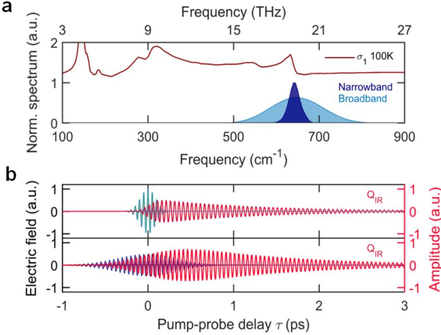
**Figure C.4.** (a) Equilibrium  $c$ -axis optical conductivity,  $\sigma_1(\omega)$ , of  $\text{YB}_2\text{Cu}_3\text{O}_{6.5}$  at 100 K ( $T > T_C$ , red solid line), along with the frequency spectra of THz probe (grey), broadband pump (light blue), and 19.2 THz narrowband pump (dark blue) pulses. (b) The amplitude of the 19.2-THz mode driven by 150 fs (upper) and 600 fs (lower) pump pulses with the same pulse energy.
