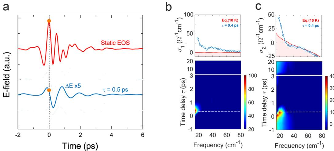
**Figure 4.18.** (a) Stationary reflected probe electric field and corresponding pump-induced electric field changes for 20 THz broadband excitations at a pump-probe delay  $\tau = 0.5$  ps. (b-c) Frequency- and time-delay-dependent pump-induced optical conductivity measured after broadband excitation at 20 THz ( $T = 10$  K, below  $T_c$ ). The white dashed lines indicate the pump-probe time delay  $\tau = 0.5$  ps.
