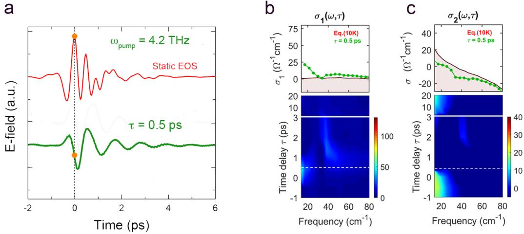
**Figure 4.20.** (a) Stationary reflected probe electric field and corresponding pump-induced electric field changes for 4.2 THz narrowband excitations at a pump-probe delay  $\tau = 0.5$  ps. (b-c) Frequency- and time-delay-dependent pump-induced optical conductivity measured after narrowband excitation at 4.2 THz ( $T = 10$  K, below  $T_c$ ). The white dashed lines indicate the pump-probe time delay  $\tau = 0.5$  ps.
