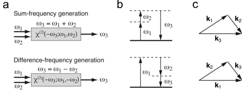
**Figure 2.2.** (a) Schematic illustration of two principle second-order nonlinear processes: sum-frequency generation and difference frequency generation. (b) Corresponding photon energy conservation. (c) Corresponding wavevectors satisfying the phase-matching condition. Adapted from [49].
