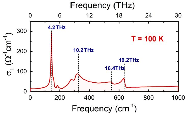
**Figure 4.3.** Real part of optical conductivity  $\sigma_1$  along c-axis of  $\text{YBCO}_{6.5}$  at 100 K (above  $T_c$ ). Four dominant modes peak at  $140 \text{ cm}^{-1}$  (4.2 THz),  $337 \text{ cm}^{-1}$  (10.2 THz),  $547 \text{ cm}^{-1}$  (16.4 THz) and  $640 \text{ cm}^{-1}$  (19.2 THz) are noted in blue and indicated with dashed lines.
