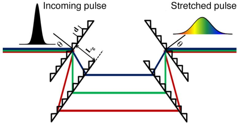
**Figure 2.12.** Schematic representation of the stretcher used in the experiment. The stretcher is made by two transmission grating pairs. The total amount of negative dispersion introduced by the stretcher is proportional to the distance  $L_g$  between the gratings constituting a pair.
