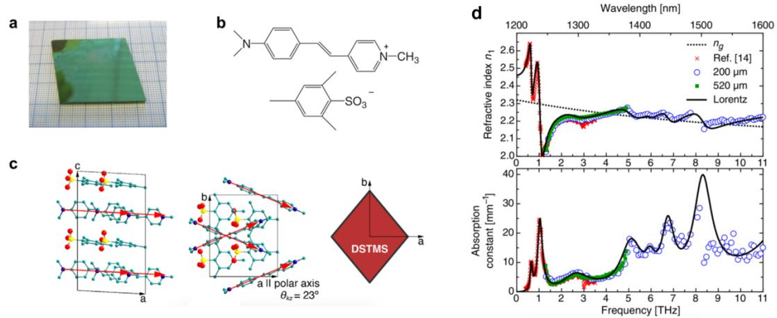
**Figure 2.10.** (a) DSTMS bulk crystal, the large surface is the (001) face. (b) Molecular structures [90] and (c) the dominant sample morphology of DSTMS [49]. (d) Terahertz refractive index and absorption of DSTMS crystals for polarization parallel to the polar a-axis. Adapted from [92].
