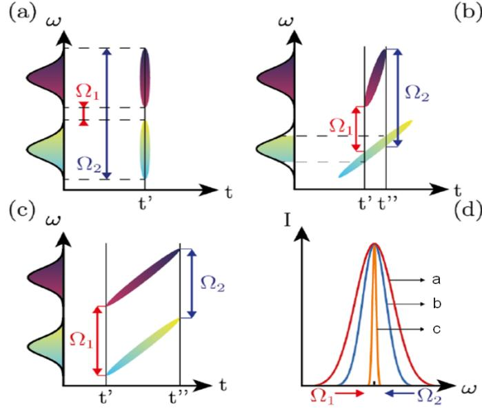
**Figure 2.8. Principle of the narrowband MIR pulse generation.** (a-c) Time-frequency Wigner distributions of the interacting NIR pulses for various chirp configurations; the THz components are generated at the difference frequency between NIR spectral frequencies at the same time delay.  $\Omega_1$  and  $\Omega_2$  are the lowest and highest MIR frequencies, respectively. (d) Corresponding MIR spectra. For configuration (a-c). Adapted from Ref. [97].
