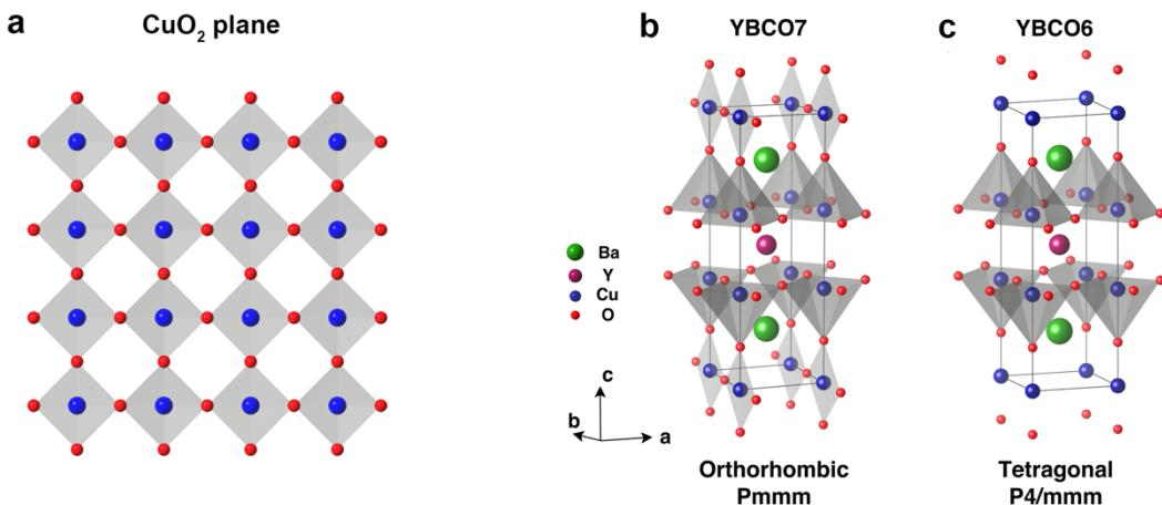
**Figure 3.5.** (a) Copper-oxygen plane in cuprates. (b) Orthorhombic structure of  $\text{YBCO}_7$  (superconductor), which has  $Pmmm$  symmetry. (c) Tetragonal structure of  $\text{YBCO}_6$  (insulator), which has  $P4/mmm$  symmetry. The octahedrons are highlighted in grey.
