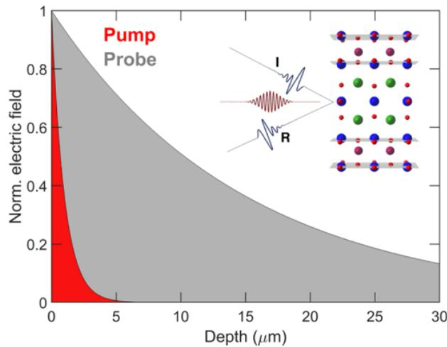
**Figure 4.7.** Penetration depth for the pump and probe beam in the experiment. The electric field of both pump (red) and probe (grey) exponential decay as a function of penetration. The inset illustrates the pump and probe beam together with the  $\text{YBa}_2\text{Cu}_3\text{O}_{6.5}$  in the horizontal plane.
