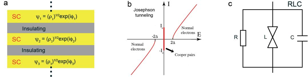
**Figure 3.7.** (a) Stacked Josephson junctions. Superconducting layers are stacked between insulating buffer layers.  $\psi_i$  is the wave function for the superconducting electrons. (b) Electron tunneling between Josephson layers. There is a  $2\Delta$  energy gap for normal electrons to tunnel through different Josephson layers, however, no energy loss for the Cooper pairs tunneling. (c) Equivalent RLC circuit model of the Josephson junctions.
