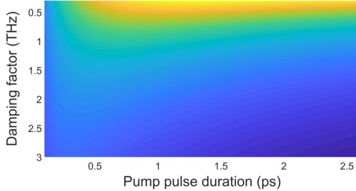
**Figure C.2** The maximum amplitude of the investigated oscillator as a function of the damping coefficient and pump pulse duration. The phonon frequency is set to be 19.2 THz. The pump pulses are set to be transform-limited.
