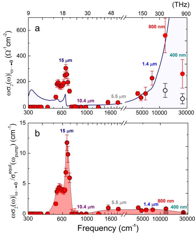
**Figure 4.23.** (a) Pump frequency dependence of the superconducting response, represented by the low-frequency limit  $\omega\sigma_2(\omega)|_{\omega\rightarrow 0}$  (red circles). The equilibrium optical conductivity,  $\sigma_1^{equil}(\omega_{pump})$ , is shown as a blue line. (b) Normalized response,  $\omega\sigma_2(\omega)|_{\omega\rightarrow 0}/\sigma_1^{equil}(\omega_{pump})$  (red circles).
