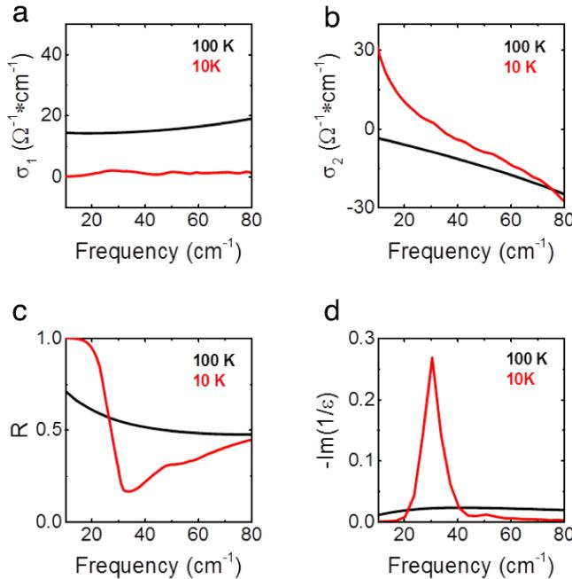
**Figure 4.2.**  $C$ -axis THz-frequency optical properties in the equilibrium superconducting ( $T < T_c$ , red curves) and normal ( $T > T_c$ , black curves) state in YBa<sub>2</sub>Cu<sub>3</sub>O<sub>6.5</sub>. **(a-b)** The real and imaginary parts of optical conductivity  $\sigma_1(\omega)$ ,  $\sigma_2(\omega)$ , **(c)** the reflectivity  $R(\omega)$ , and **(d)** the energy loss function  $-\text{Im}(1/\varepsilon)$  are reported.
