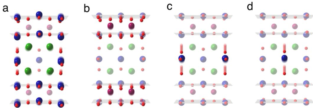
**Figure 4.4.** Atomic displacement along the normal coordinates of four dominant IR-active optical phonons polarized along c-axis in  $\text{YBa}_2\text{Cu}_3\text{O}_{6.5}$  at (a) 4.2 THz, (b) 10.1 THz, (c) 16.4 THz, and (d) 19.2 THz. The  $\text{CuO}_2$  layers are highlighted in grey and transparency is applied to quasi-stationary atoms.
