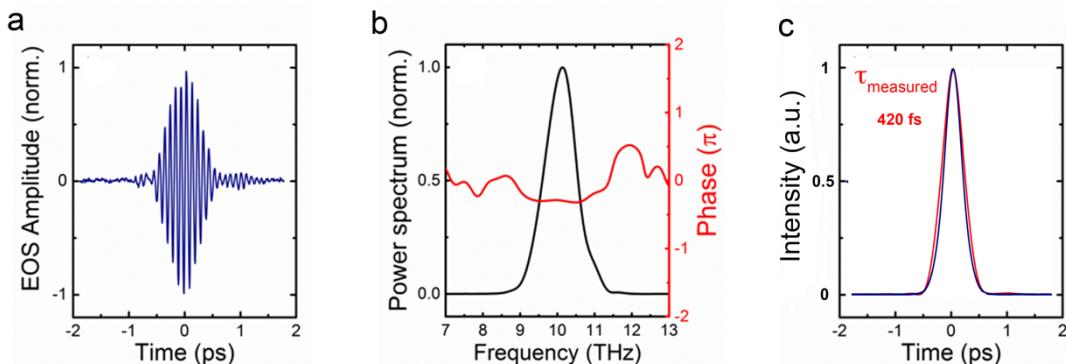
**Figure 2.15.** (a) The THz electric field generated by DFG in a 480  $\mu\text{m}$  thick DSTMS crystal as detected via electro-optic sampling in a GaSe crystal of 100  $\mu\text{m}$  thickness. (b) Corresponding power spectrum (black) and spectral phase (red). (c) Retrieved pulse duration from the EOS measurement (red) and the constructed transform limit pulse from the measurement (blue).
