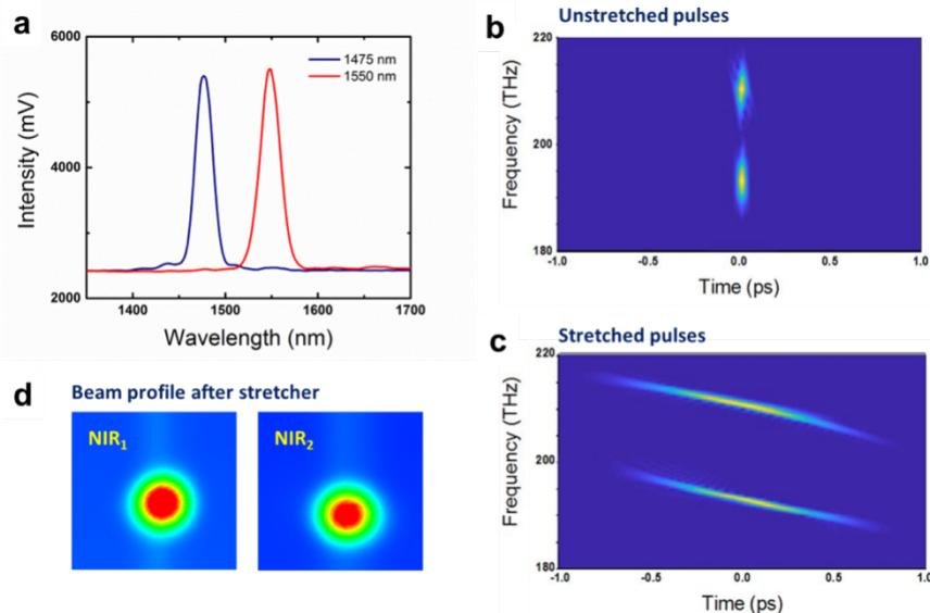
**Figure 2.13.** (a) Spectra intensity of the two NIR beams with central wavelength at 1475 and 1550 nm and  $\sim 30$  nm bandwidth as the pump and signal in the DFG process. (b-c) Wigner map as a function of frequency and time for the two NIR beams before (b) and after (c) the transmission grating stretcher. (c) depicts the two stretched pulses with roughly the same GDD (the slope of the frequency-time trace). (d) Beam profile after the stretcher measured with CCD camera for NIR light.
