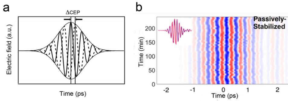
**Figure 2.19.** (a) Example of carrier-envelope phase shift. (b) CEP stability characterization of narrowband pulses. Due to the passive stabilization in the difference frequency generation process, the recorded electro-optical sampling over 240 minutes (4 hours) with negligible drift proves the generated pulses to be CEP stable. Inset: EOS traces measured with 1-hour interval.
