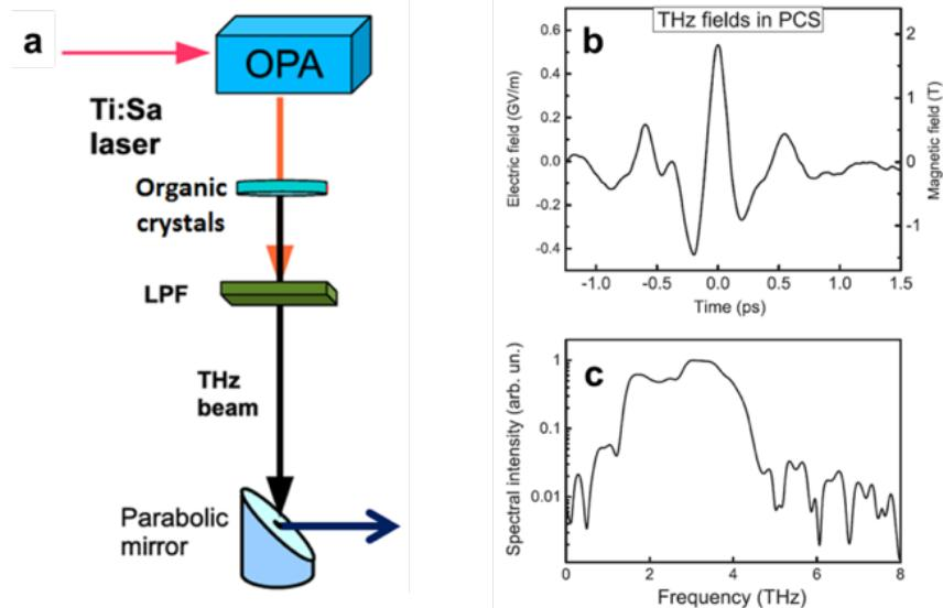
**Figure 2.5. (a)** Tabletop terahertz source based on the partitioned DSTMS. The crystal is pumped by an optical parametric amplifier (OPA). The THz beam is separated from the residual pump by a low-pass filter (LPF). THz electric field **(b)** and corresponding spectrum **(c)** obtained by optical rectification in a patterned DSTMS crystal structure. Adapted from Ref. [69].
