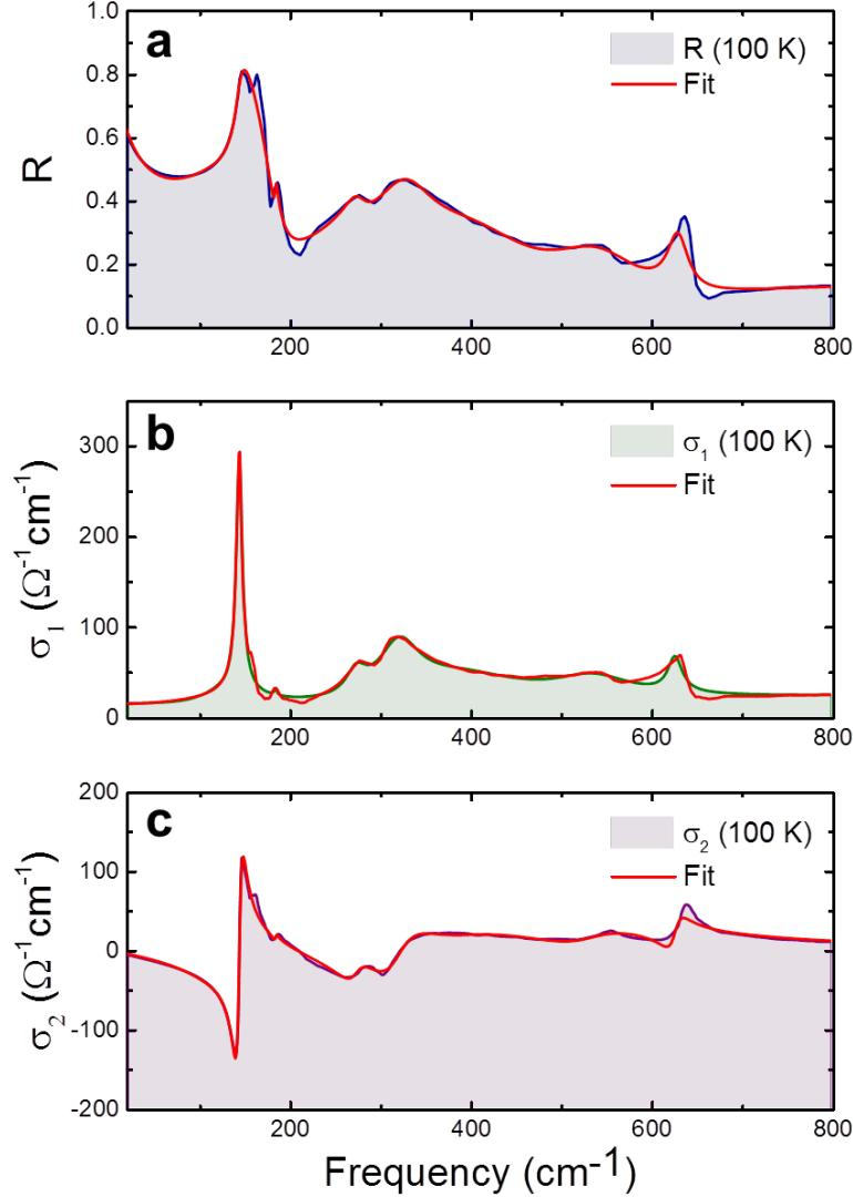
**Figure 4.8.** Equilibrium c-axis optical properties of YBCO<sub>6.5</sub> at 100 K fitted with Drude-Lorentz model. The colorful curves with shadows are (a) reflectance, (b) real part and (c) imaginary part of optical conductivity. The red curves are the fits with one set of fitting parameters which are listed in Table 4.1.
