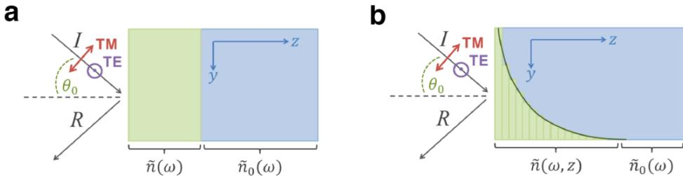
**Figure D.3.** Different models for penetration depth mismatch in data analysis. **(a)** Single-layer model. The material is modeled as a single excited layer on an unperturbed bulk. **(b)** Multi-layer model. The system is modeled as a multilayer, with the pumped volume described as a stack of thin layers with the  $z$ -independent refractive index. The refractive index decays exponentially into the material. Figures are taken from [202].
