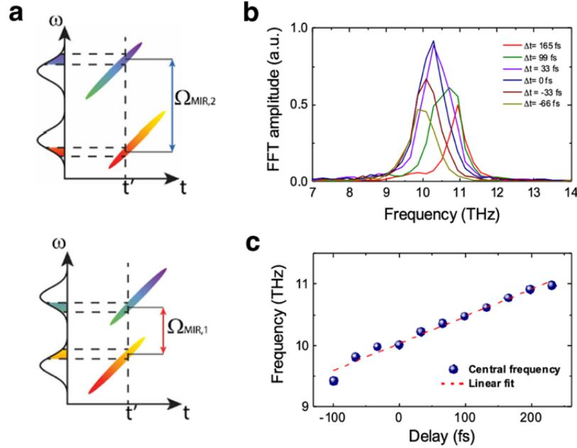
**Figure 2.16.** (a) Schematic explanation of the relationship between the delay of the two stretched NIR beams and the central frequency of generated MIR-THz pulses [97]. (b) Normalized Fourier transform amplitude of the generated THz transient around 10 THz at different time delays of the two interacting NIR beams. (c) The central frequency of the generated THz transient as a function of time delay.
