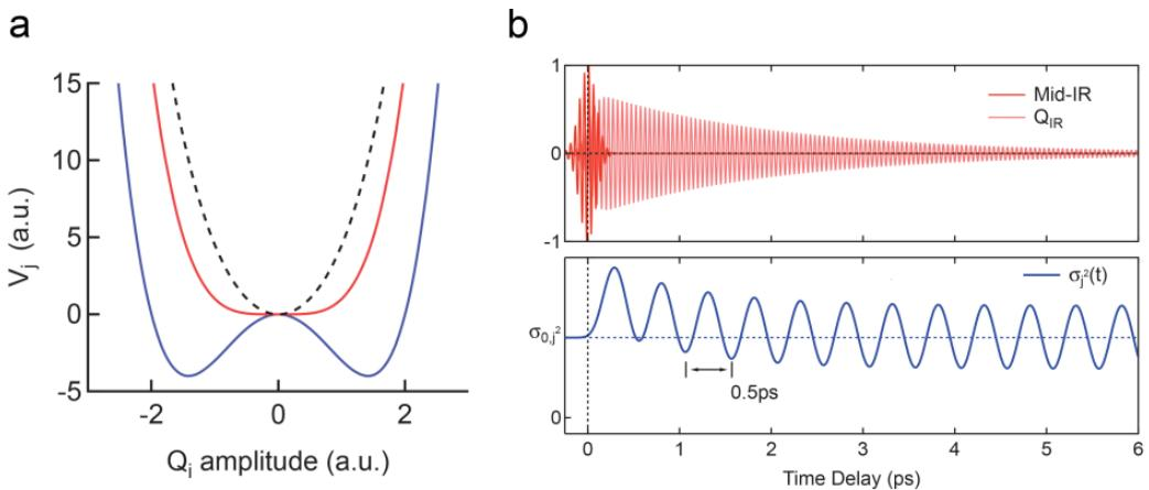
**Figure 1.2.** (a) The energy potential of the coupled mode through quartic coupling. It is deformed to be softened (red) or stiffened into an unstable double well potential. (b) Instead of displacing the crystal lattice, the variance of the coupled mode  $\sigma_j^2 = \langle Q_j^2 \rangle$  is oscillating at twice the frequency of the coupled mode [17].
