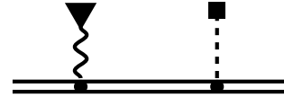
FIG. 1. Feynman diagram corresponding to the hypothetical NP contribution to the g factor of a bound electron. The double line represents the bound electron, the wavy line terminated by a triangle denotes a photon from the external magnetic field, and the dashed line terminated by a square denotes a scalar boson from the nuclear neutrons.
