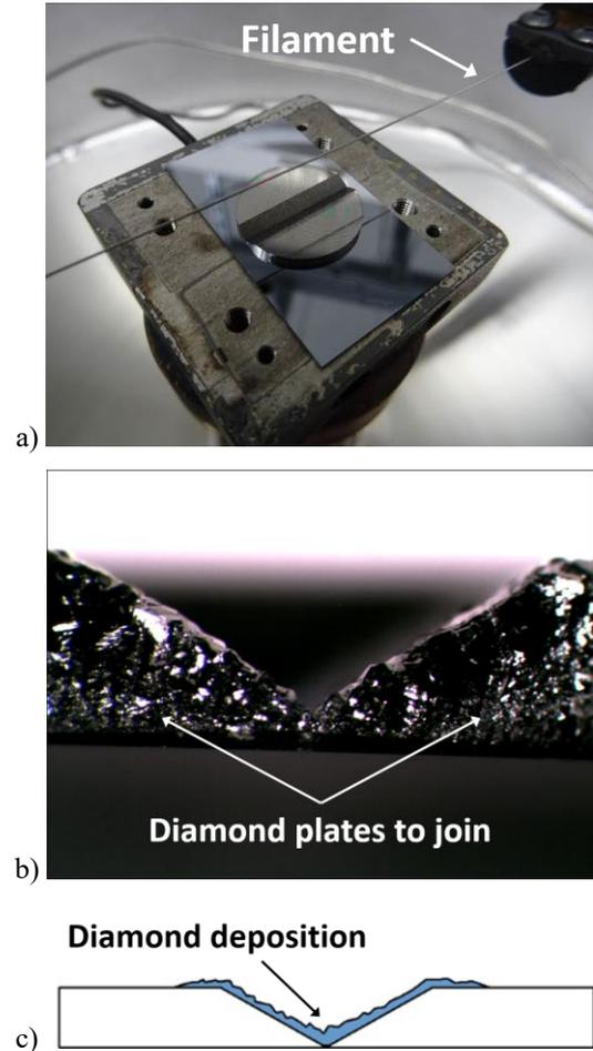
Fig. 3. Diamond plates ready to be joined by the hot filament method (a) and resulting compound (b), better described by the model in (c). The position of the filament in (a) is not adjusted in height.
