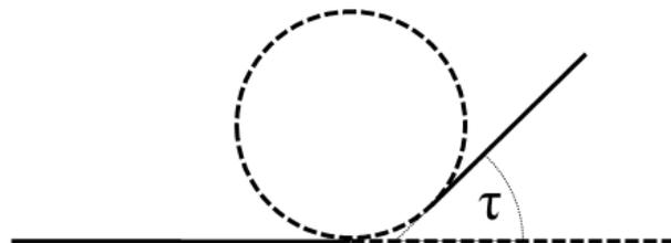
Fig. 5: Tangents on beginning and end of a bend
