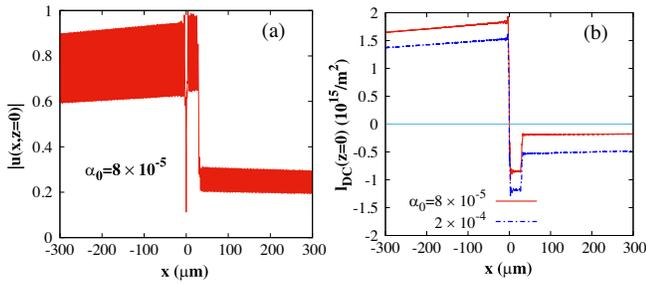
FIG. 3. Snapshot of the displacement field at the GGG surface  $|u|$  [(a)] and phonon spin density [(b)], pumped by a YIG wire at the origin under FMR and modulated by a second YIG wire at  $30 \mu\text{m}$ .
