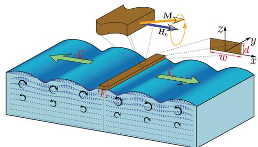
FIG. 1. Surface-phonon pumping by one magnetic nanowire (brown) on top of the acoustic insulator (blue). A static magnetic field  $\mathbf{H}_0$  applied in the  $\vec{x}$  direction saturates the magnetization. The pumped Rayleigh SAWs by the nanowire FMR propagate and rotate in opposite directions at the two sides of the nanowire as indicated by the green and black arrows, respectively.
