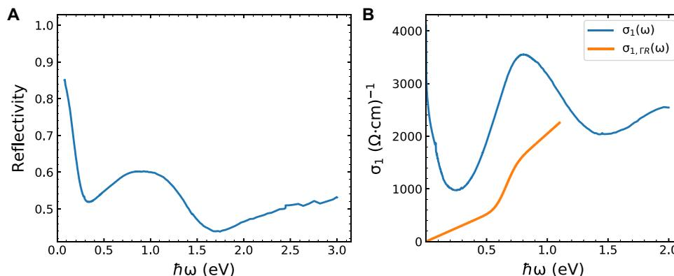
**Fig. 4. Reflectivity and optical conductivity.** (A) Measured reflectivity of RhSi. (B) Optical conductivity determined by reflectivity measurements and Kramers-Kronig analysis (blue curve). The Drude peak is used to infer that the scattering time has value  $\tau = 8.6$  fs. The orange curve represents the optical conductivity from the  $\Gamma$  and  $R$  nodes alone (34).
