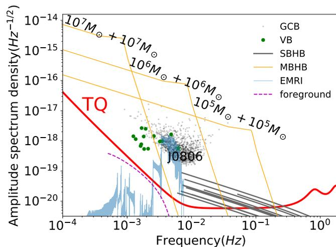
**Figure 1.** Expected astrophysical sources for TianQin. In this plot, the information of the detector response is included in the signal strain of each source and the instrumental noise (the solid red curve) is approximated by dividing  $S_n(f)$  by 10/3, which accounts for the geometric configuration of TianQin, as well as the location- and polarisation-sensitive response in the low frequency limit.
