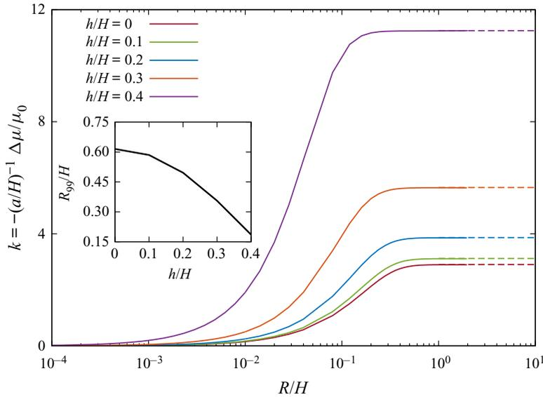
FIGURE 4. Variations of the correction factor of the hydrodynamic mobility as defined by (3.3) versus  $R/H$  for various values of  $h/H$ . Horizontal dashed lines correspond to the correction factor near two infinitely large disks as given by (3.4). Inset: Evolution of  $R_{99}/H$  versus  $h/H$ , where  $R_{99}$  is defined such that  $k(R_{99}/H) = 0.99k_{\infty}$ , for which the correction factor near infinitely large disks is almost recovered.
