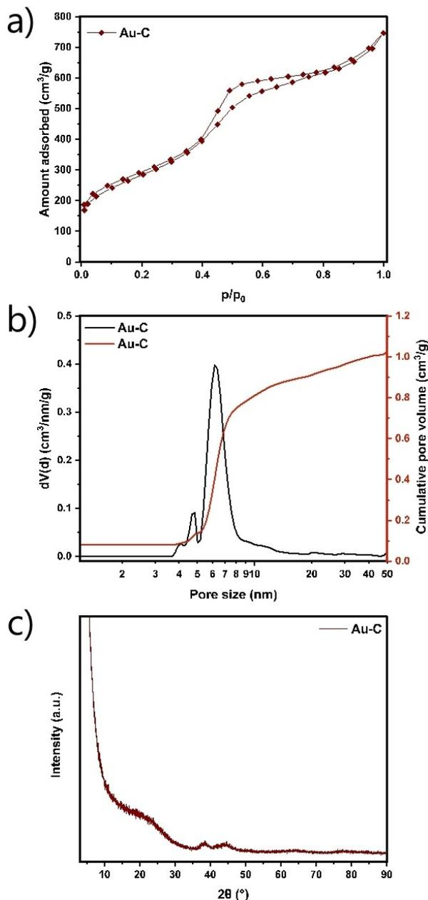
**Figure 1.** a)  $N_2$  physisorption isotherm (at  $-196^\circ\text{C}$ ) with the corresponding b) differential and cumulative pore size distribution plots calculated with QSDFT ( $N_2$  on carbons with slit/cylindrical/spherical pores at 77 K, adsorption branch kernel), and c) powder XRD pattern of Au–C.
