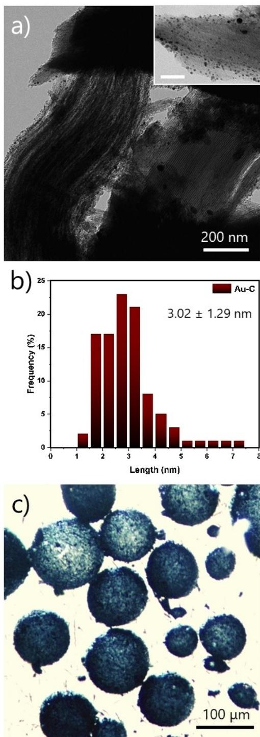
**Figure 2.** a) TEM images of the Au–C catalyst (length of scale bar in the insert is 50 nm), b) AuNP size distribution with the average NP size in Au–C catalyst, and c) microscopy image of Au–C–PFC Pickering emulsion with 2 vol.% PFC in water.
