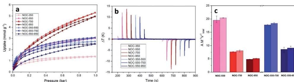
Fig. 4 (a) Carbon dioxide physisorption isotherms at 273 K, (b)  $\text{CO}_2$  thermal response adsorption and desorption measurements at 1 bar and  $25 \text{ }^\circ\text{C}$ , and (c) integrated adsorption and desorption (left bar and right bar, respectively) temperature peak area normalized by the mass and the total pore volume from Ar physisorption of NOC-Xs and NOC-X-Ys.
