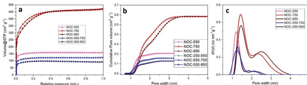
Fig. 3 (a) Argon physisorption isotherms (87 K), (b) corresponding cumulative pore volume distribution, and (c) differential pore size distribution calculated with QSDFT (argon on carbons with cylindrical/spherical pores at 87 K) of NOC-*X*s and NOC-*X*-*Y*s.
