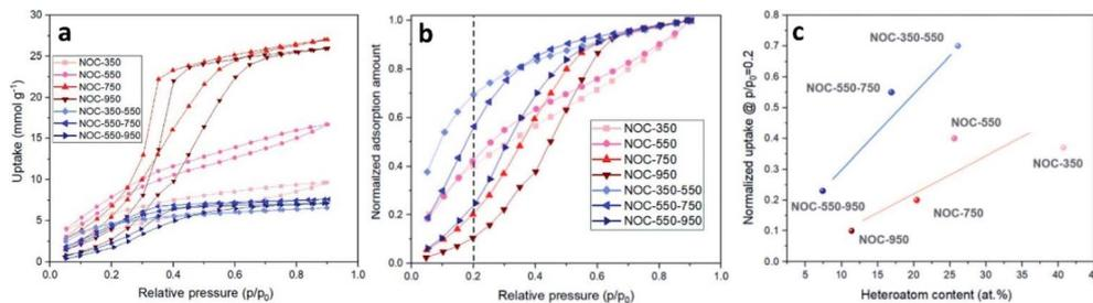
Fig. 5 (a) Water vapor physisorption isotherms at 298 K, (b) normalized amount adsorbed relative to the maximum H<sub>2</sub>O uptake at 298 K, and (c) the normalized uptake at relative pressure  $p/p_0 = 0.2$  as a function of the nitrogen and oxygen content of NOC-Xs and NOC-X-Ys from XPS.
