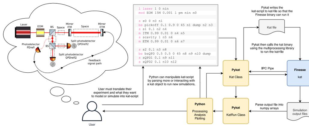
**Fig. 1.** A schematic of the typical workflow a user has with PYKAT. Initially the user must have a concrete idea of the physical setup they want to model, and then express this setup in kat-script. This script can then be loaded into a PYKAT object which allows the user to run multiple simulations, perform more complex analyses, and generate plots. Behind the scenes, PYKAT will seamlessly setup and call the FINESSE binary to run the required simulations.
