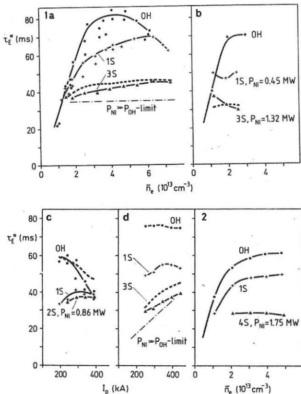
Fig. 1: Density and current scaling of the global energy confinement time of deuterium discharges. S = number of NI-sources
