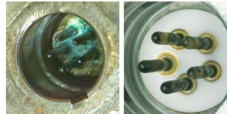
198 Fig. 7 (left) 5 pin electrical feed through showing the corrosion 199 at the Molybdenum pins (see also fig. 4 [2]). (right) 200 Refurbished feed-through.
