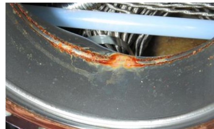
211 Fig. 8 Rust at both sides of a welding seam in a pump duct.
