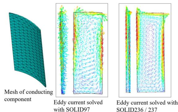
Fig. 3. Comparison of the eddy currents calculated with SOLID97 and SOLID236 / 237.
