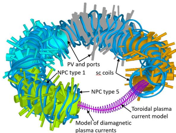
Fig. 6. The  $360^\circ$  EM model expanded from sector EM model with plasma currents, PV and multiple ports (different colors for the PV and ports in different sectors).
