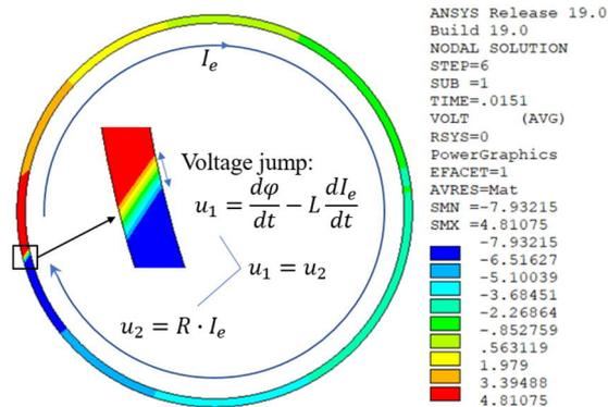
Fig. 5. Explanation of the voltage drop along the eddy current loop solved by SOLID236 / 237,  $\varphi$  is the magnetic flux,  $I_e$  is the eddy current,  $L$  is the self-inductance of the eddy current loop,  $R$  is the resistance of eddy current loop.
