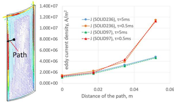
Fig. 4. Comparison of the skin effect considered by different element types ( $\tau$  is the excitation current decay time constant).
