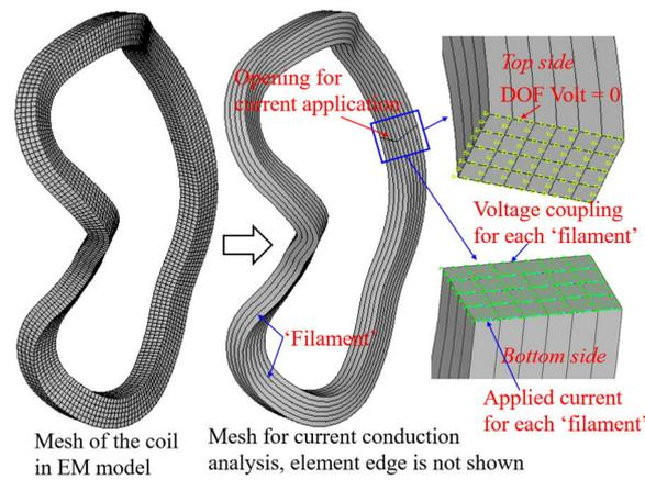
Fig. 2. Modelling and BC for current conduction analysis of W7-X non-planar coil (NPC) type 1 (close to the middle of one W7-X sector).
