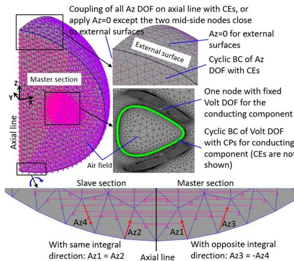
Fig. 1. Specific boundary conditions for sector EM model and the explanation of cyclic BC with CEs.
