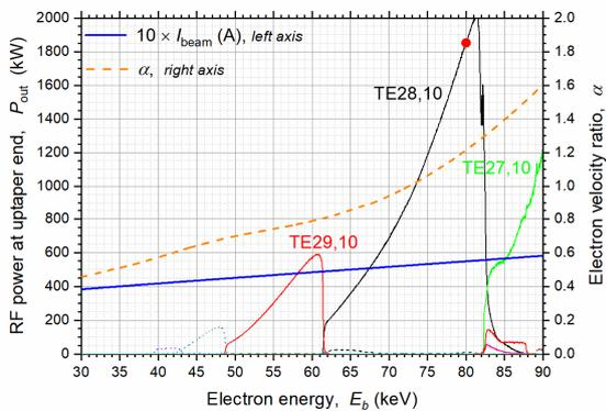
Fig. 2. Multi-mode (45 modes) simulation of the gyrotron beam-wave interaction, showing the power of different modes versus the kinetic energy of the electron beam. The nominal operating point is marked by the red point. The electron velocity ratio and the beam current are also shown.
