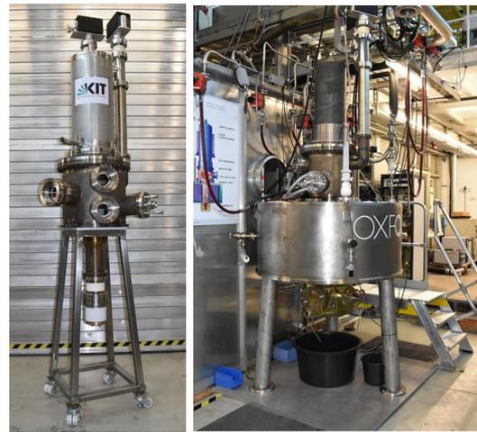
Fig. 10. The first configuration of the 1.5 MW 140 GHz short-pulse gyrotron before (left) and after (right) installation at the KIT gyrotron test stand.
