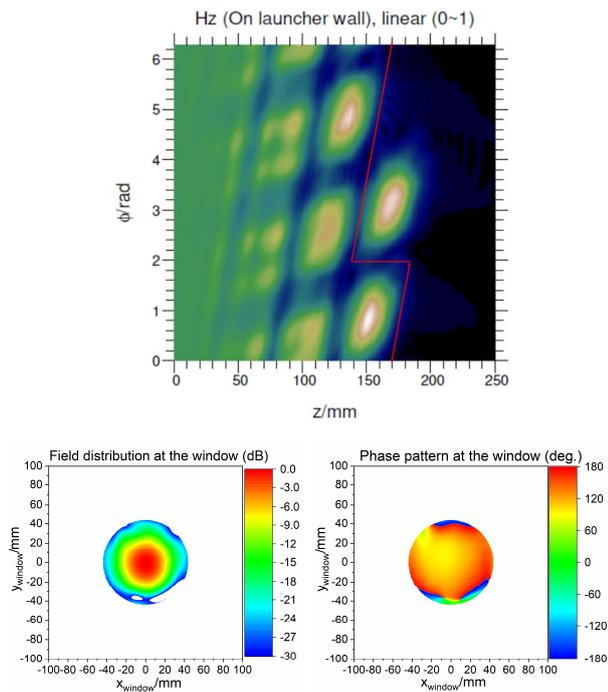
Fig. 6. Top: simulated RF field amplitude on the launcher wall. The launcher cut is shown by the red line. Bottom: Simulated amplitude (left) and phase (right) of the RF field distribution at the window.
