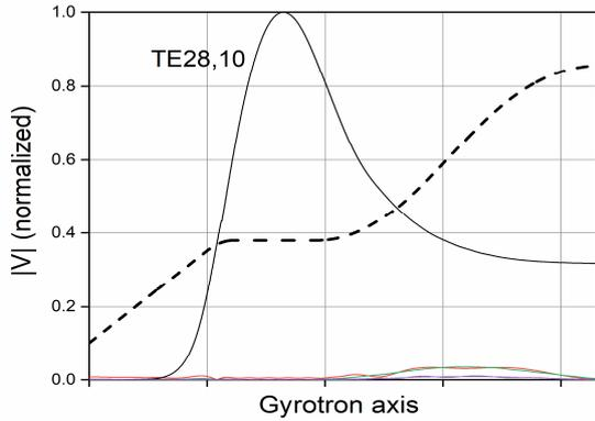
Fig. 1. Contour of cavity and non-linear uptaper of the 1.5 MW prototype along the gyrotron axis (thick dashed curve) and calculated mode conversion along the axis, shown by the normalized amplitude of the main  $TE_{28,10}$  mode (black curve) and of the spurious modes (colored curves).
