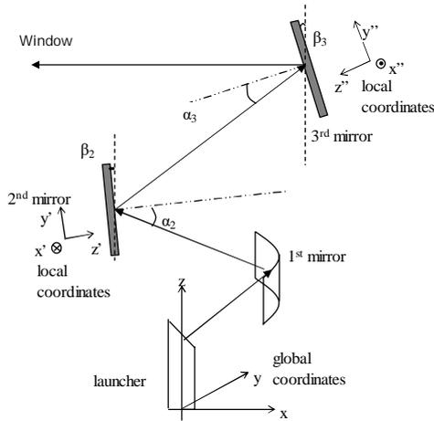
Fig. 5. Schematic of the quasi-optical system of the 1.5 MW gyrotron.
