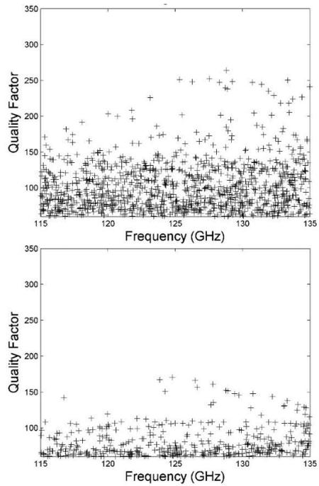
Fig. 4. Cold-cavity calculation of frequencies and quality factors  $Q$  of resonant parasitic modes with  $Q > 60$  in the existing beam tunnel of the 1 MW gyrotron at W7-X (top) and in the alternative beam tunnel design for the 1.5 MW gyrotron (bottom). The improvement offered by the alternative design is apparent.
