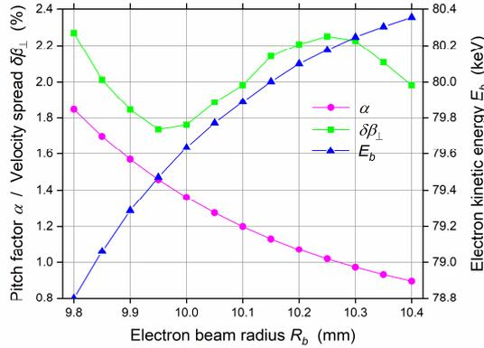
Fig. 3. Electron gun simulation at 55 A beam current and 82 kV accelerating voltage with *Ariadne*: calculated electron velocity ratio  $\alpha$ , rms transverse velocity spread  $\delta\beta_{\perp}$ , and electron kinetic energy  $E_b$  as functions of the electron beam radius. (The nominal beam radius of the 1.5 MW gyrotron is 10.1 mm.)
