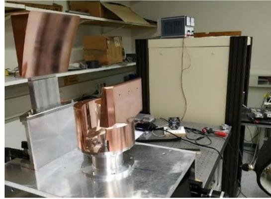
Fig. 8. Assembly of the quasi-optical system for the low-power measurements.
