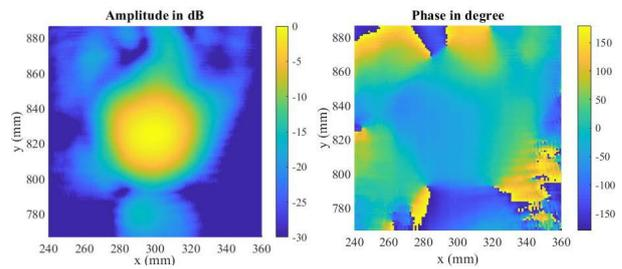
Fig. 9. Low-power measurements with the complete quasi-optical system: amplitude (left) and phase (right) of the RF field at the window plane.
