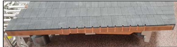
Fig. 4: Apertures machined in TM2H for the integration of the pop-up array of Langmuir probes.
