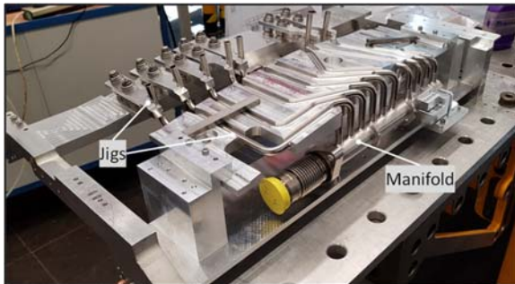
Fig. 6. Example of the manufacturing process of the sub-group manifold + pipes for TM1V.
