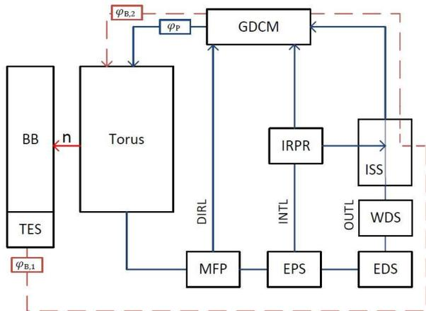
Fig. 2: Simplified layout of the DEMO fuel cycle including tritium pathways from the reactor exhaust (straight blue line) and breeding blanket (dashed red line).
