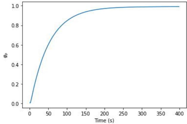
Fig. 3: Step change response of the Dirl and Intl starting from D<sub>2</sub> operation to the nominal exhaust tritium content of  $z_T=0.485$  reaching  $\varphi_P = 0.99$  after 350s.
