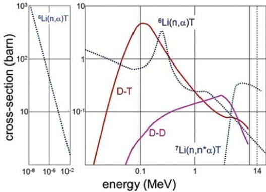
Fig. 1: Cross sections of the  ${}^6\text{Li}$  and  ${}^7\text{Li}$  breeding reactions as a function of the impacting neutron energy. D-D and D-T cross-sections as a function of the plasma energy are reported as well. Figure is taken from [13].
