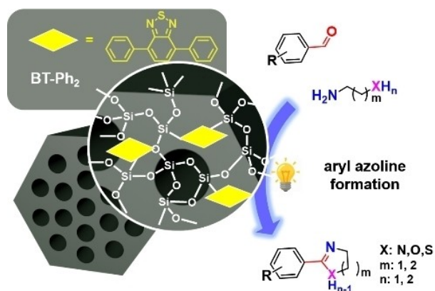
Scheme 1. Illustration of the design concept of the photocatalytic mesoporous organosilica and their application in aryl azoline formation via addition of aryl aldehydes and amine derivatives.
