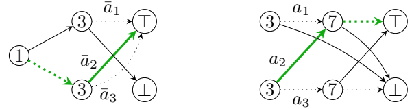
Figure 2. Given variable intervals x_1, x_3 \in \mathcal{I}^p, x_7 \in \mathcal{I}^q with p < q , the BDD from Figure 1 is split into two sub-BDDs. For consistency between sub-BDDs, active paths must agree on the copy-arc pairs (\bar{a}_1, a_1) , (\bar{a}_2, a_2) and (\bar{a}_3, a_3) . The two paths marked with green arcs correspond to the path marked in Figure 1.
