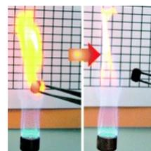
**Figure 3.** Photographs of noble carbon foams resisting a welding flame at 1000 °C. Reproduced with permission from reference<sup>34</sup>
