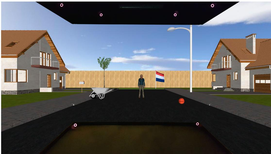
**Figure 1.** An example of the CAVE set up. Six of the ten infrared motion tracking cameras are visible, four at the top of the three projector screens and two in the bottom corners. The scene displays the virtual agent in the centre of the street scene, along with the six target objects (lamppost, basketball, flag, tree, letterbox, and wheelbarrow).
