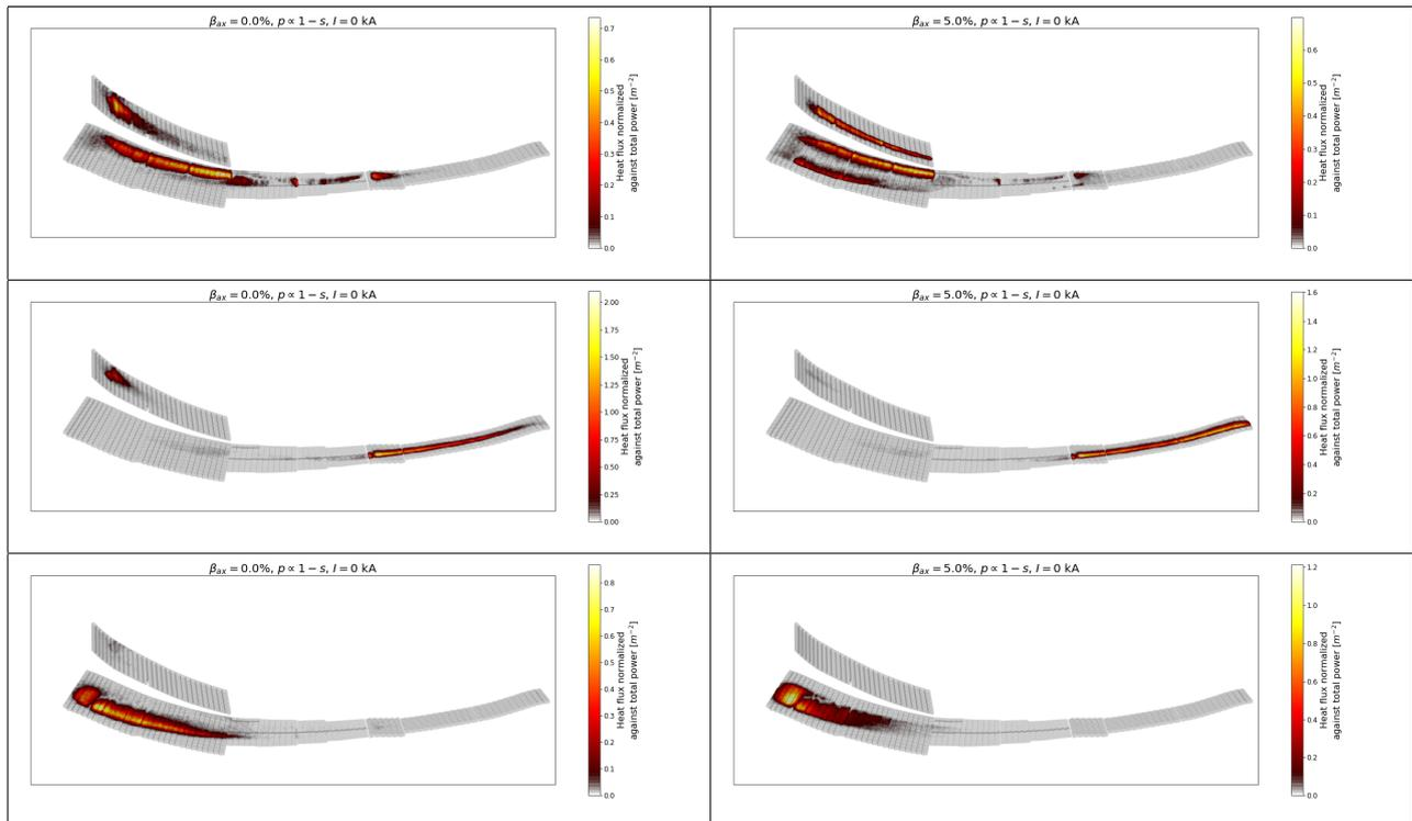
Figure 2: Simulated heat-loads normalized against the total power flow into the scrape-off layer (in unit  $\text{m}^{-2}$ ) for standard (top), high-iota (middle) and low-iota (bottom) configuration in vacuum (left) and 5% on-axis plasma beta (right)
