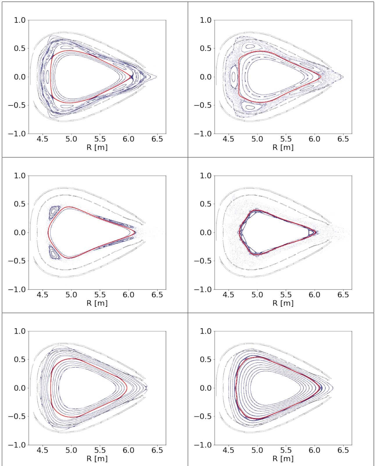
Figure 1: Magnetic topology for standard (top), high-iota (middle) and low-iota (bottom) configuration in vacuum (left) and 5% on-axis plasma beta (right). The red line indicates the flux-surfaces used to seed the heat-load test packets for the heat-load distributions in figure 2
