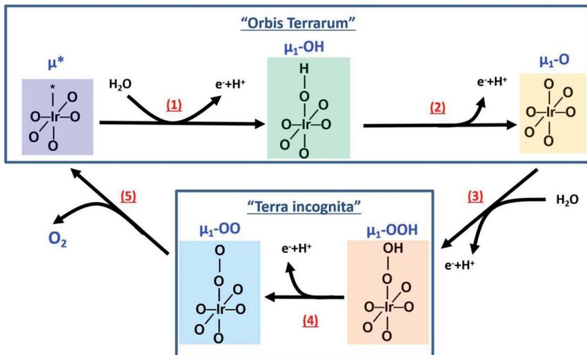
Fig. 7 Schematic representation of the simplified reaction pathway. The upper part shows the intermediates that can be considered to be known according to the *operando* spectroscopy and literature available (“Orbis Terrarum”). The bottom part represents part of the reaction pathway that has not been probed experimentally (“Terra incognita”) until the current ResPES experiments presented in this work.
