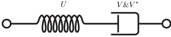
FIG. 5. Diagram corresponding to the passive odd Maxwell model. The “&” refers to a parallel connection of an odd and an even component of the same type.
