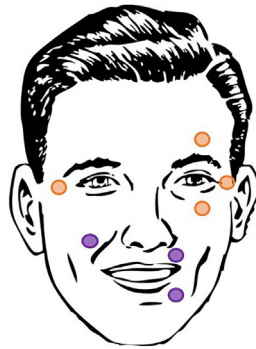
Figure 9. EOG and EMG electrodes placement for the recording of eye (orange) and mouth (purple) movements, respectively
