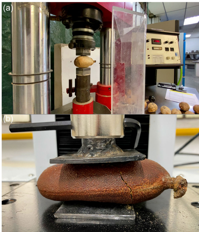
FIGURE 4 (a) Babaçu nut ( At. speciosa ) being tested at the Universal tester TONI COMP III, at the Associação Brasileira de Cimento Portland (ABCP), São Paulo, Brazil. (b) Jatobá ( H. courbaril ) being tested by the custom universal mechanical tester at the Laboratory of Plant Anatomy at the Institute of Biosciences, University of São Paulo. A fracture can be seen in the fruit.
