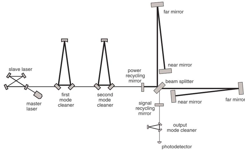
**Figure 1.** A schematic of the optical layout of GEO 600 showing the input laser system, the two sequential mode cleaners followed by the dual-recycled Michelson interferometer and an output mode cleaner. The output photodiode is mounted outside the vacuum system.
