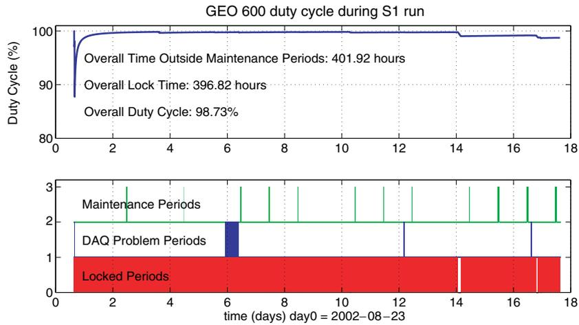
**Figure 6.** The duty cycle of GEO over the S1 run. In the calculation of the duty cycle, maintenance periods that were used are counted as dead time, DAQ down-time is counted as out-of-lock, and the DAQ error period is included as lock-time.
