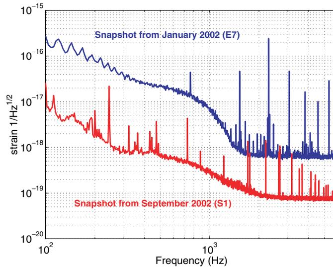
**Figure 5.** Snapshots of calibrated error-point spectra from GEO at two different times in 2002.
