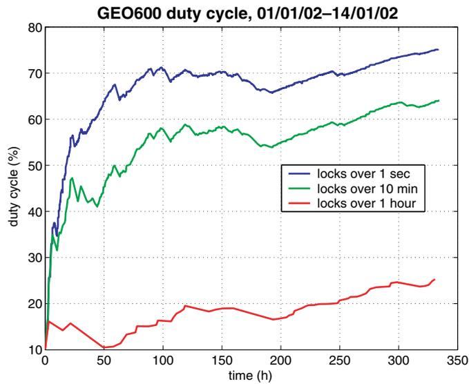
**Figure 3.** The cumulative duty cycle of GEO calculated between 1 and 14 January 2002.
