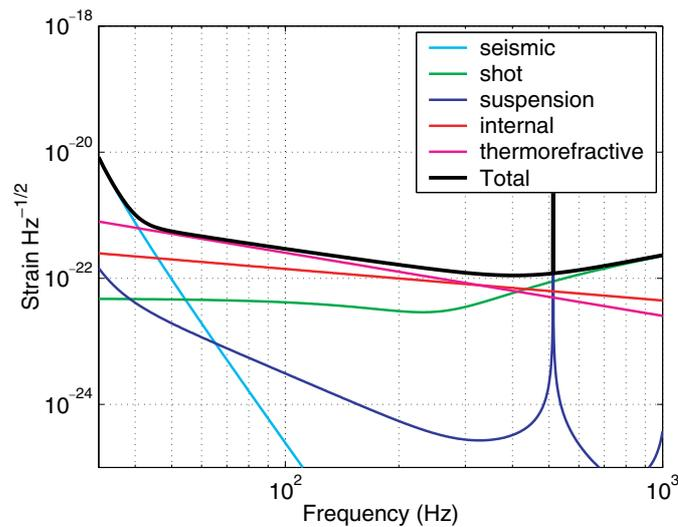
**Figure 2.** Modelled noise sources present in GEO 600 that contribute to the shown design sensitivity curve (total). The internal noise curve represents the thermal noise present in the test masses. The suspension noise curve consists mainly of the thermal noise present in the silica fibres of the monolithic suspensions.
