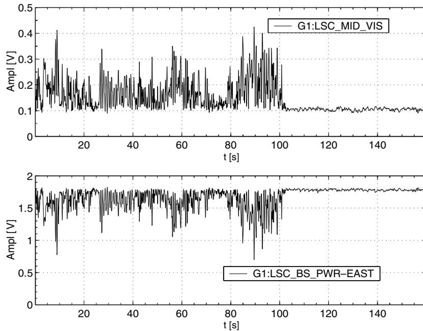
**Figure 4.** Time-series plots of the dark fringe power (upper trace) and power in the PR cavity (lower trace) with and without Michelson auto-alignment switched on.
