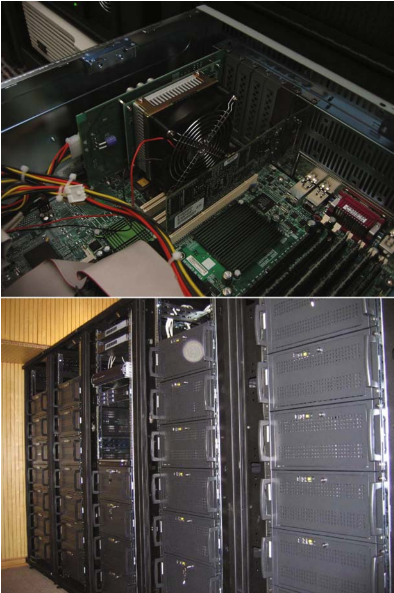
Fig. 15.2. Top: interior of a node showing a GRAPE-6A card (note the large black fan) and an Infiniband card. Bottom: the GRACE cluster at ARI. The head node and the 14 Tbyte raid array are visible on the central rack. The other four racks hold a total of 32 compute nodes, each equipped with a GRAPE-6A card and MPRACE cards
