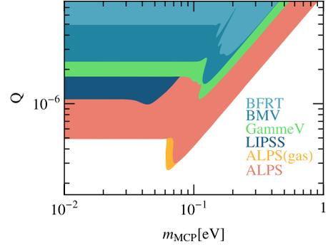
**Fig. 6.** 95% C.L. exclusion limits for mini-charged particles in models with a hidden photon. We have taken  $e_h = e$ , so  $Q = \chi$ . (For interpretation of the references to colour in this figure, the reader is referred to the web version of this Letter.)
