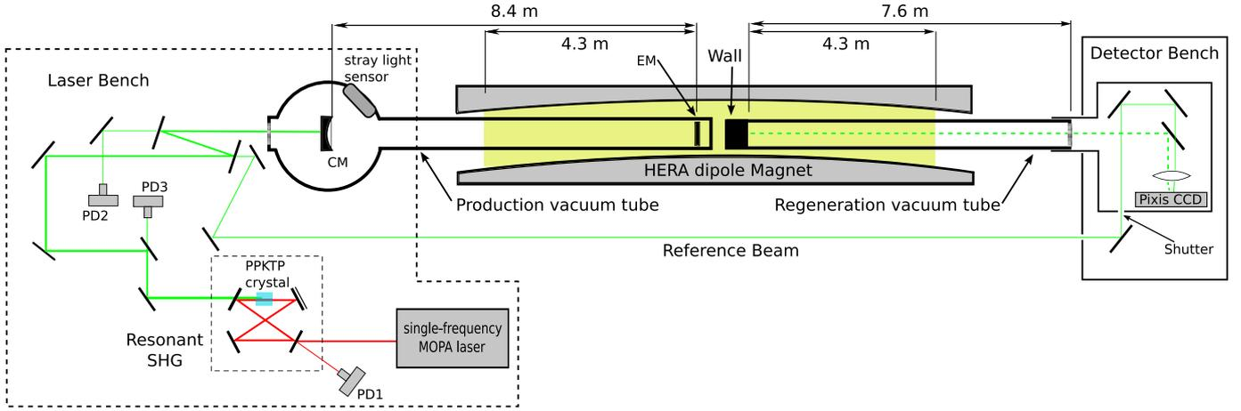
**Fig. 1.** Schematic view of the ALPS LSW experiment. See the text for a description. (For interpretation of the references to colour in this figure, the reader is referred to the web version of this Letter.)
