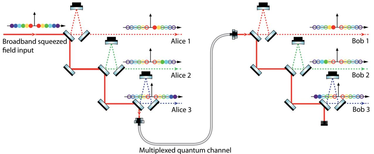
FIG. 4: (Colour online) Distribution of sideband fields of a squeezed field for  $N = 3$  EPR channel multiplexing. For each EPR channel a pair of filter cavities and a pair of frequency shifted local oscillators (not shown) are required.
