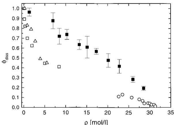
**Fig. 5.** Photodissociation quantum yields of iodine in  $\text{CO}_2$  (■:  $\lambda_{\text{exc}} = 532$  nm at 323 K, this work; ○:  $\lambda_{\text{exc}} = 590$  nm at 298 K [10]; △:  $\lambda_{\text{exc}} = 581$  nm at 330 K [6]; □:  $\lambda_{\text{exc}} = 694$  nm at 314 K [5]).
