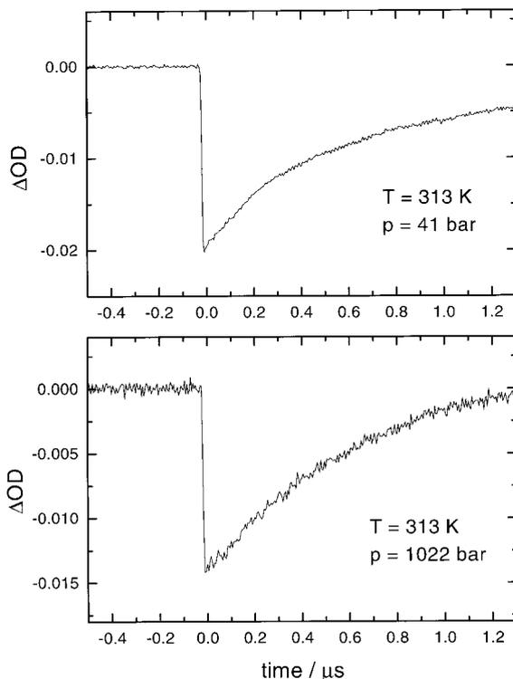
**Fig. 3.** Recombination of iodine in xenon at 41 and 1022 bar after photodissociation with laser pulses at 532 nm (observation wavelength: 514 nm;  $T = 313$  K).
