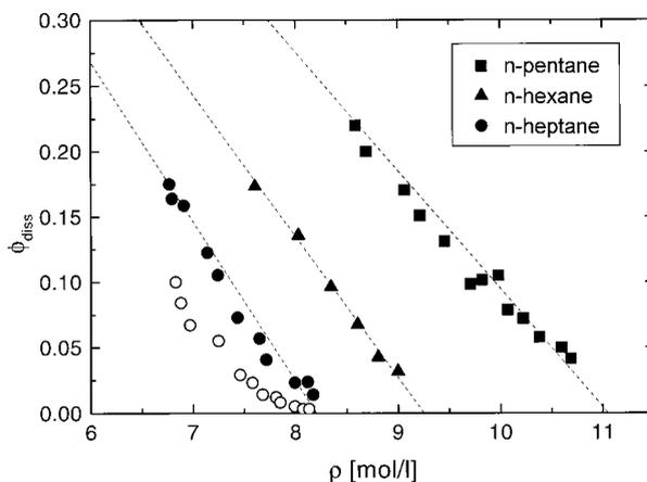
**Fig. 4.** Photodissociation quantum yields of iodine in compressed liquid  $n$ -alkanes at 298 K (full symbols: excitation at 532 nm, this work; open circles: excitation at 590 nm, from [10, 12]; dashed lines intercept at  $\phi_{\text{diss}}(\rho = 0) = 1$ ).
