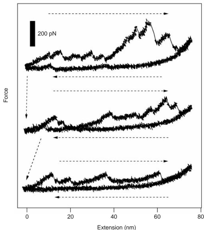
**Figure 2** Consecutive force–extension curves, obtained using an atomic force microscope, from pulling on a freshly cleaved abalone nacre surface. Rupture events, with a sawtooth appearance, are visible in each of the curves. The surface was not touched between pulls, strong evidence that some refolding took place, possibly of domains in lustrin A. The approach and retract curves show hysteresis, indicating that the rupture events dissipate energy.
