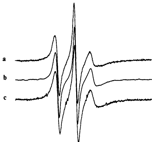
FIG. 8. ESR spectra of the 14-PGSL phosphatidylglycerol spin label in aqueous dispersions of lipid extracts of: a , cucumber; b , pea; and c , lettuce thylakoids. Total scan width = 100 gauss; T = 18^\circ\text{C} .
