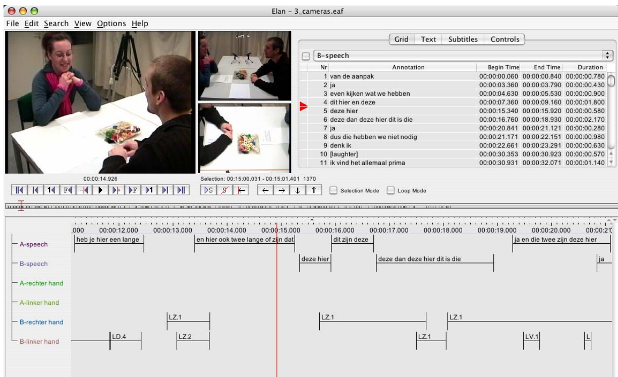
Figure 3 shows a typical screen layout for ELAN. Multiple synchronized video streams are embedded, different viewers for the annotations are available. In the lower part the time line viewer presents the annotations, created on user-defined tiers, time aligned with media time. In the upper right part the grid viewer renders the annotations of one tier in a more readable, tabular way.
