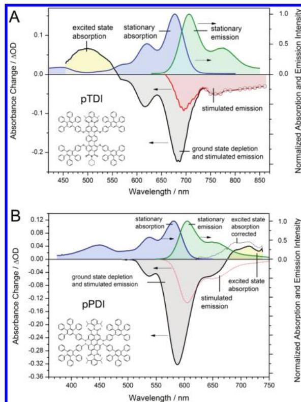
**Figure 4.** Transient absorption spectra of pTDI and pPDI. The transient absorption band ( $S_1 \rightarrow S_n$ ) is blue-shifted for pTDI and well-separated from the stimulated-emission band and STED de-excitation beam wavelength (780 nm) used. The excited-state absorption band of pPDI overlaps with the stimulated-emission spectrum; at the STED beam wavelength (700 nm), strong  $S_1 \rightarrow S_n$  absorption occurs.
