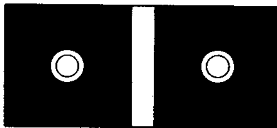
Fig. 3. Stimuli used to determine equibrightness curves. In Expt. I the concentric circles were absent when the data of Fig. 4 were collected, but were present in both monocular fields of both test and comparison fields for Fig. 5; in Expt. II, a circle was present in only one monocular field of both test and comparison fields. The visual angles subtended were: circular disks, 3^\circ ; concentric circles, 2^\circ in diameter and 3' in thickness.
