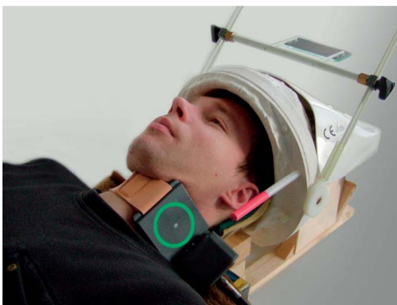
Figure 1. RF coil setup used for the perfusion experiment, here demonstrated with one of the authors as a volunteer. It consists of a 6-cm diameter circular surface coil for labeling the blood in either the left or right CCA and a 24-cm diameter circularly polarized helmet coil for brain imaging.
