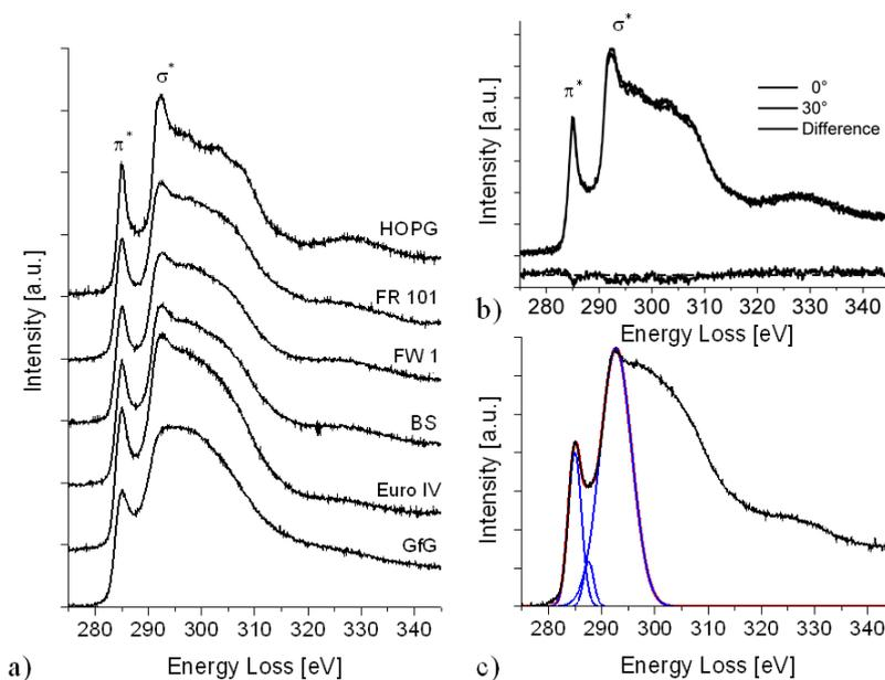
**Fig. 1** a) EELS measurements on the soot and carbon black materials, b) verification of magic angle conditions, c) fitting procedure to determine the  $sp^2/sp^3$  hybridization ratio
