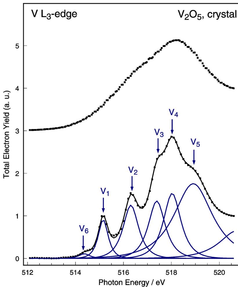
Fig. 2 (left) V L<sub>3</sub>-edge of V<sub>2</sub>O<sub>5</sub> measured with an energy resolution of 1 eV (upper) and 0.08 eV (lower), respectively. 6 resonances are obtained by deconvolution of the lower spectrum.
