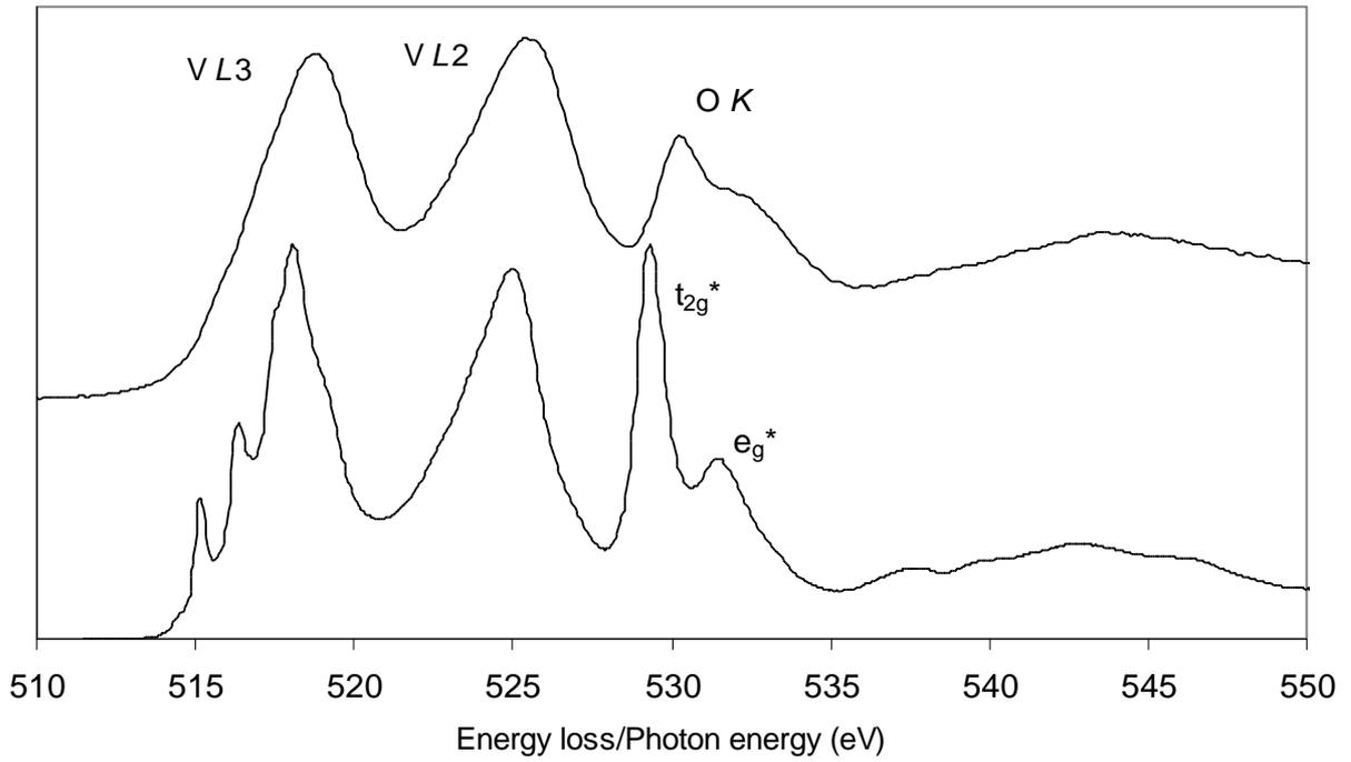
Fig. 1 (upper) ELNES and NEXAFS of V<sub>2</sub>O<sub>5</sub> with an energy resolution of 1 and 0.08 eV respectively.
