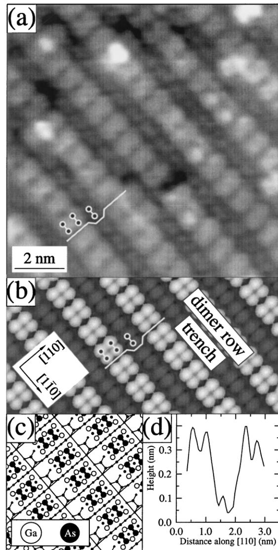
FIG. 2. (a) Filled-state STM image acquired with a sample bias of  $-2.1$  V measuring  $11\ \text{nm} \times 11\ \text{nm}$ , (b) simulated STM image of the  $\beta_2$  structural model using a filled-state bias of  $0.3$  V below the valence band maximum, (c)  $\beta_2$  structural model, and (d) height cross section across a dimer trench along the  $[110]$  direction extracted from the STM image shown in (a).
