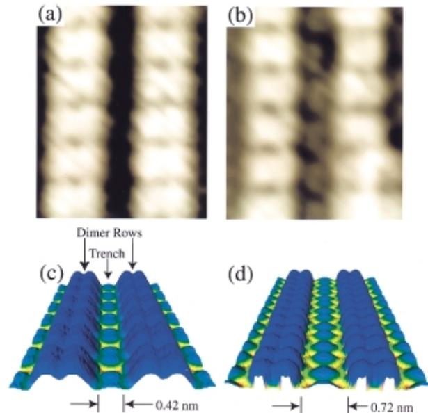
FIG. 3 (color). (a),(b)  $2.8 \text{ nm} \times 4.4 \text{ nm}$  filled-state STM images of the same area acquired with sample biases of  $-3.0$  and  $-2.1$  V, respectively. (c),(d) Simulated STM images using filled-state biases of 1.1 and 0.3 V below the valence band maximum, respectively.
