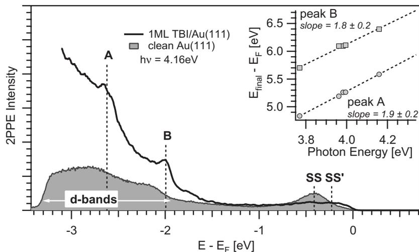
**Figure 3.** (a) One-color 2PPE spectrum of 1 ML TBI/Au(111). A comparison with the pure Au(111) signal (gray-shaded) reveals two molecule-induced states, labeled A and B, on top of the Au d-band contributions. The inset shows the final state energy of both peaks (energy of the emitted electrons with respect to  $E_F$ ) as a function of photon energy. Both peaks scale with twice the photon energy, indicating that both peaks originate from occupied initial states in the 2PPE process.
