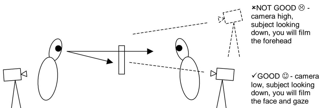
Side view of task set-up: camera low so as to capture speaker's gaze.
